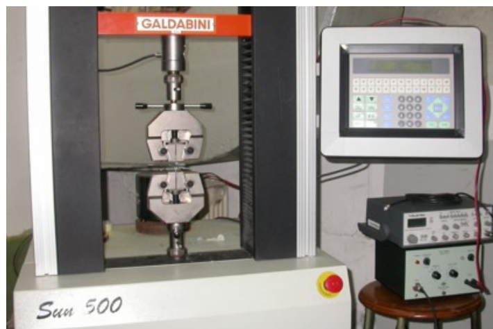
Figure 4.4 – Galdabini test machine
