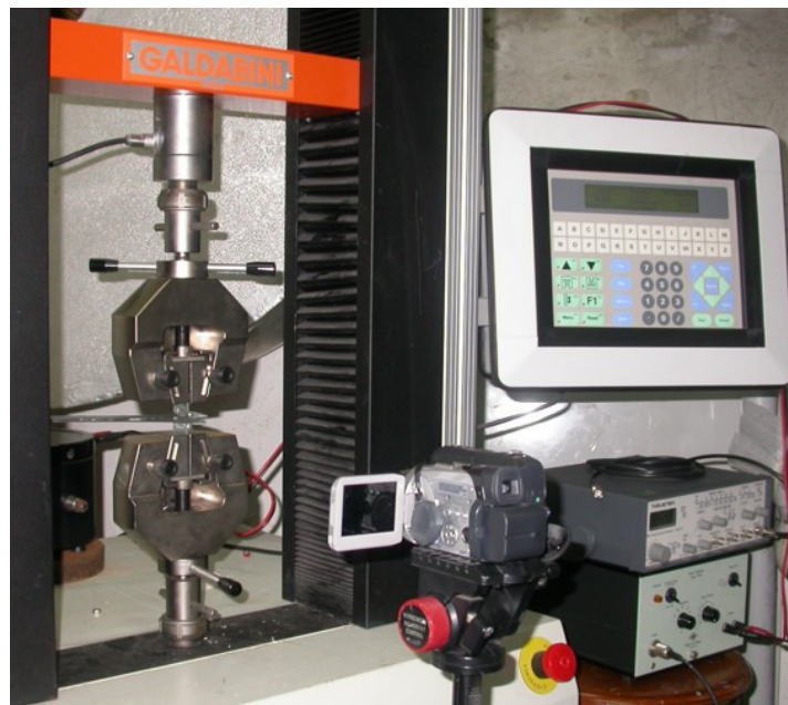
Figure 4.5 – Camcorder used to follow the propagation of the crack
