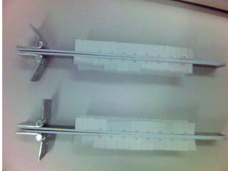
Figure 4.8 – Specimens for the DCB test
