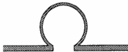
Figure 35- Layout of a single loop inductor
