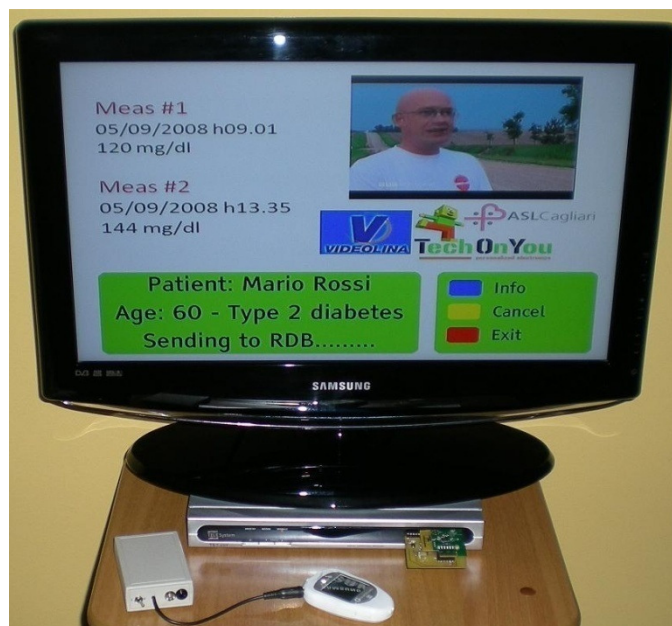
Figure 8.13: Picture of the Xlet sending two acquired glucometer measurements to the RDB.
