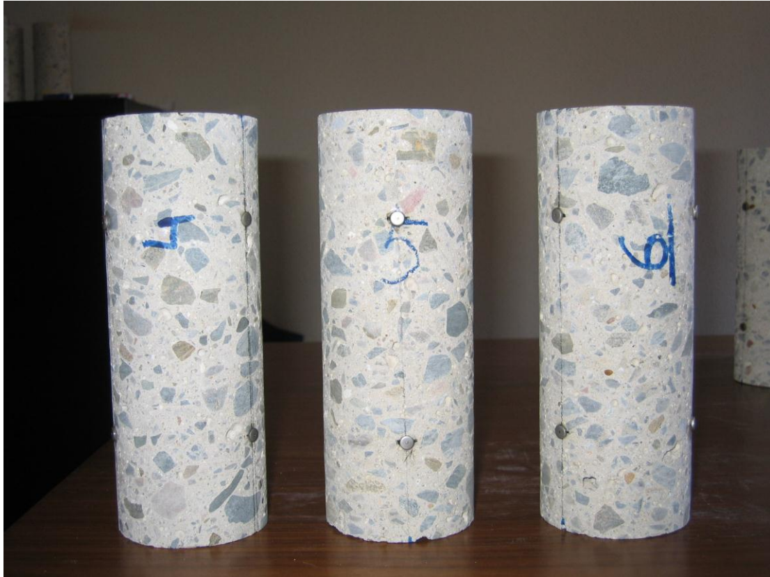
Fig. 39 - Cylinder specimens made with 50% of coarse and fine recycled aggregates + 50% naturals
