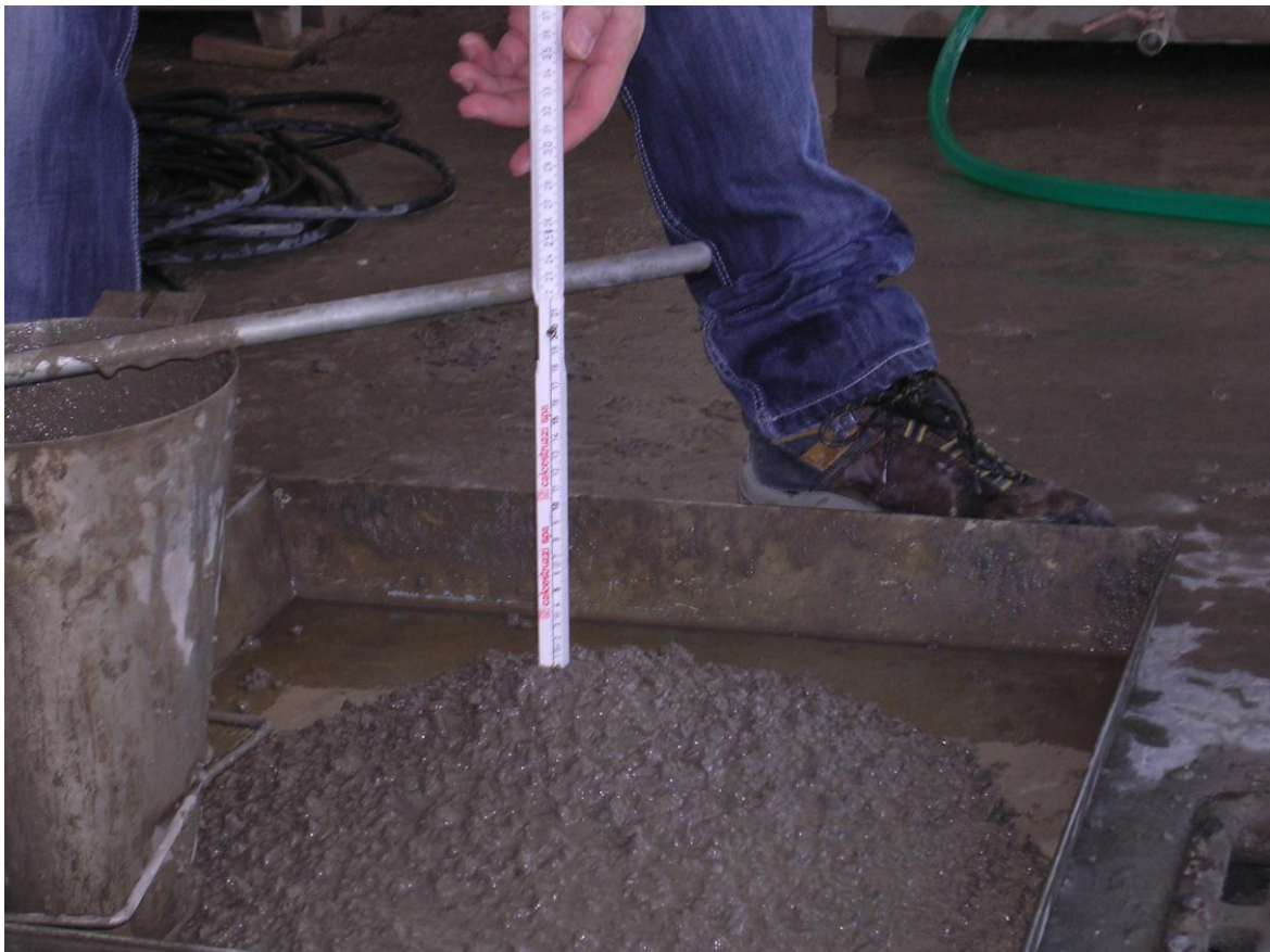
Fig. 8 - Slump 100% coarse and fine recycled aggregates, 30' - 1RC
