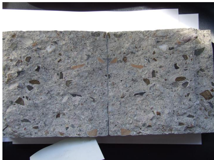
Fig. 33 - Specimen after tensile test, 100% of coarse recycled aggregates
