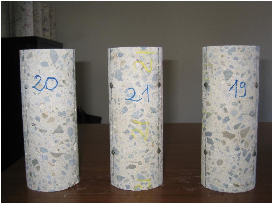
Fig. 42 - Cylinder specimens made with 50% of coarse recycled aggregates + 50% naturals
