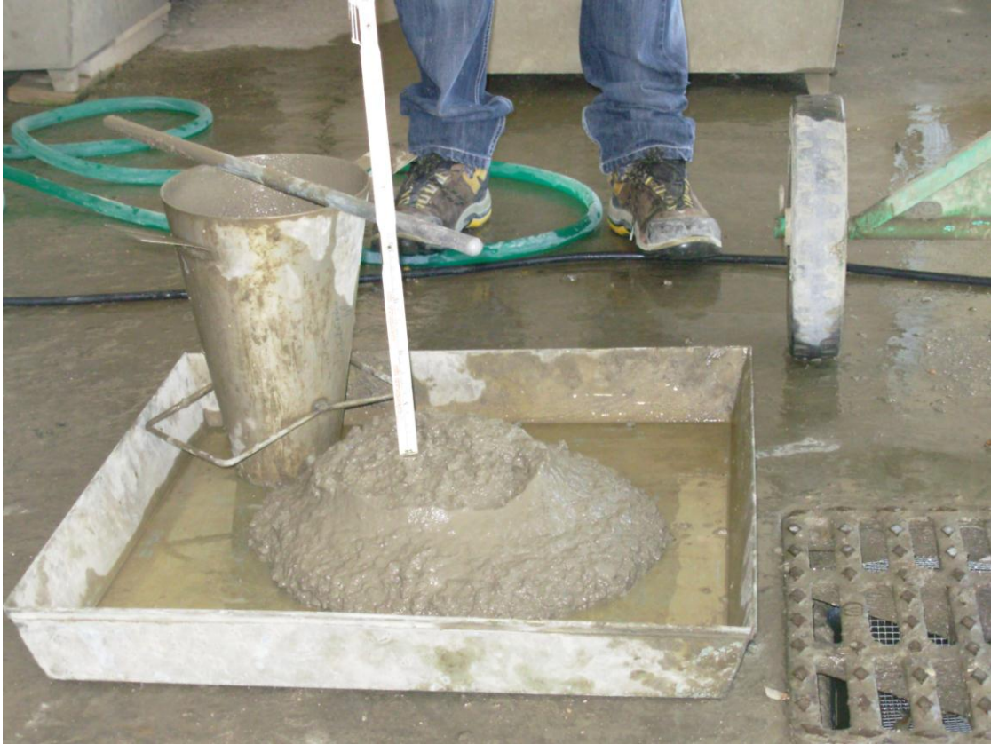
Fig. 9 - Slump 100% coarse recycled aggregates, fine totally natural , 5' - 5RC
