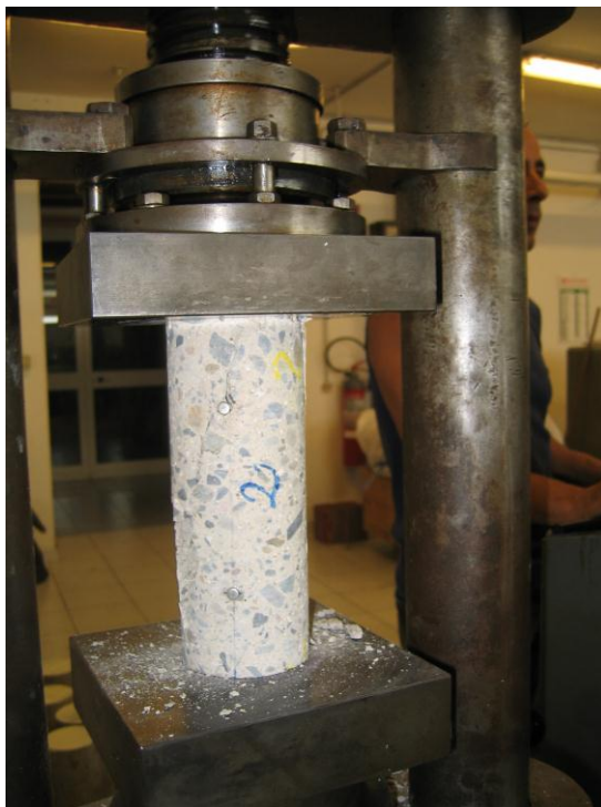
Fig. 24 - Compressive test on specimen made with 80% of coarse and fine recycled aggregates + 20% naturals
