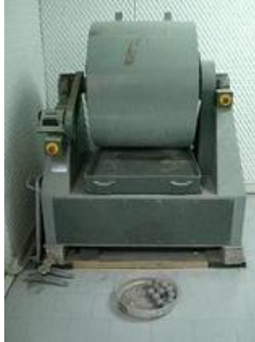
Fig. 10 – Los Angeles testing machine
