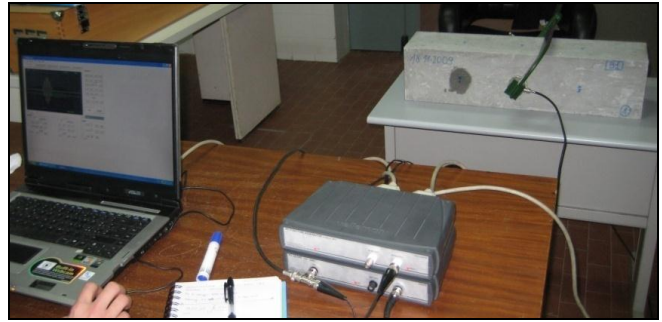
Fig. 48 - Experimental Set-up Scheme. 1) PC. 2) Signal Generator. 3) Oscilloscope. 4) Transducers. 5) Specimen
