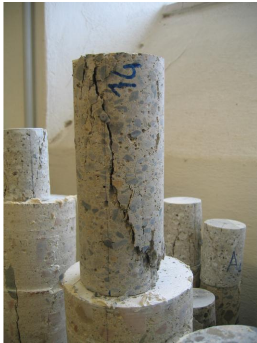
Fig. 23 - Compressive test on specimen made with 100% of coarse and fine recycled concrete
