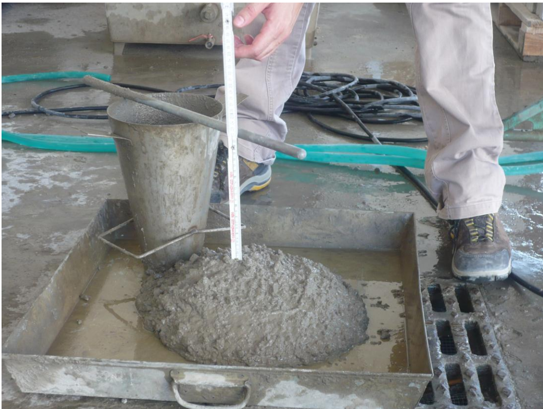
Fig. 2 - Slump 80% coarse and fine recycled aggregates + 20% coarse and fine natural aggregates, 30' - 2RC
