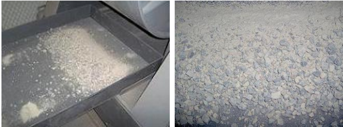
Fig 11 – Crushing of recycled aggregates after Los Angeles test
