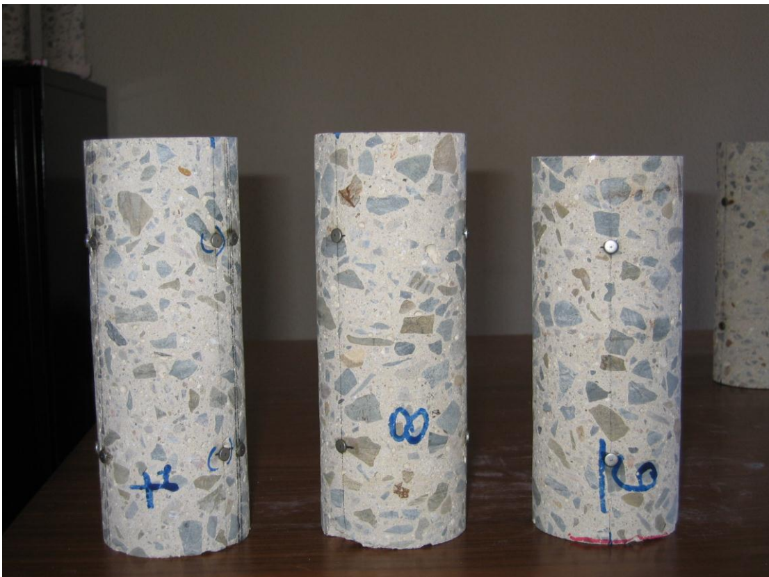
Fig. 40 - Cylinder specimens made with 20% of coarse and fine recycled aggregates + 80% naturals
