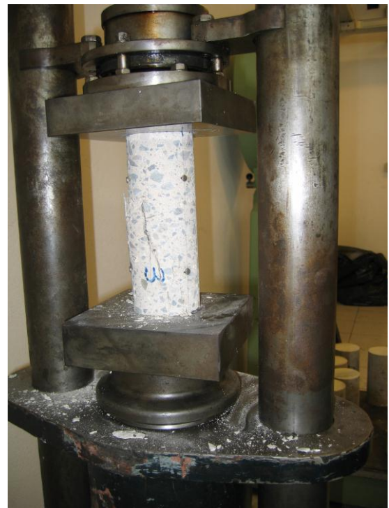
Fig. 24 - Compressive test on specimen made with 80% of coarse and fine recycled aggregates + 20% naturals
