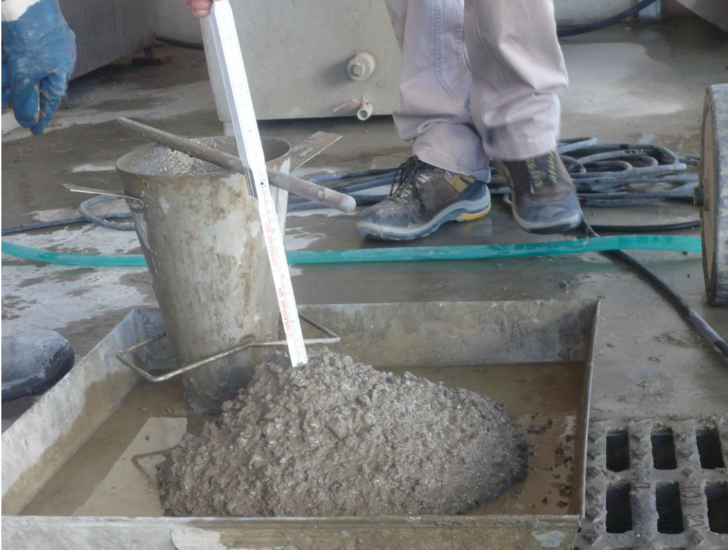
Fig. 1 - Slump 80% coarse and fine recycled aggregates + 20% coarse and fine natural aggregates, 5' - 2RC
