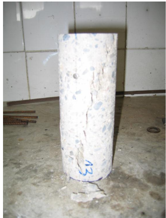
Fig. 26 - Compressive test on specimen made with 100% of coarse recycled concrete
