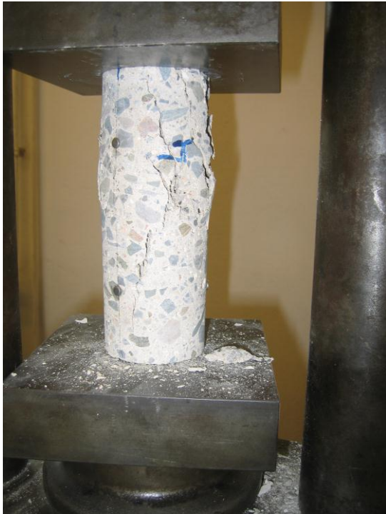
Fig. 25 - Compressive test on specimen made with 50% of coarse and fine recycled aggregates + 50% naturals
