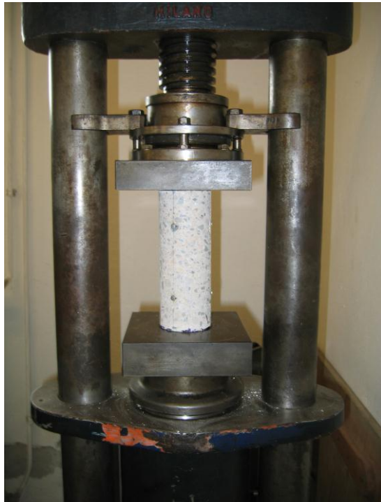
Fig. 26 - Compressive test on specimen made with 100% of coarse recycled concrete
