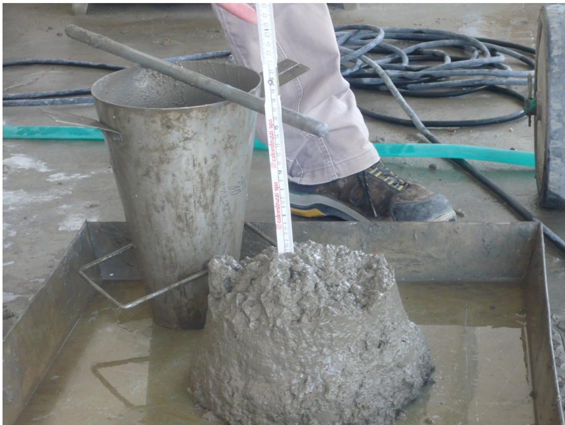
Fig. 4 - Slump 50% coarse and fine recycled aggregate + 50% coarse and fine natural aggregates, 30' - 3RC
