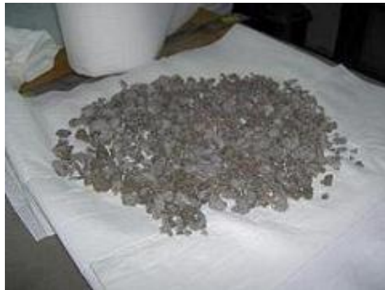
Fig. 9 – Saturated surface dry condition of the recycled aggregates
