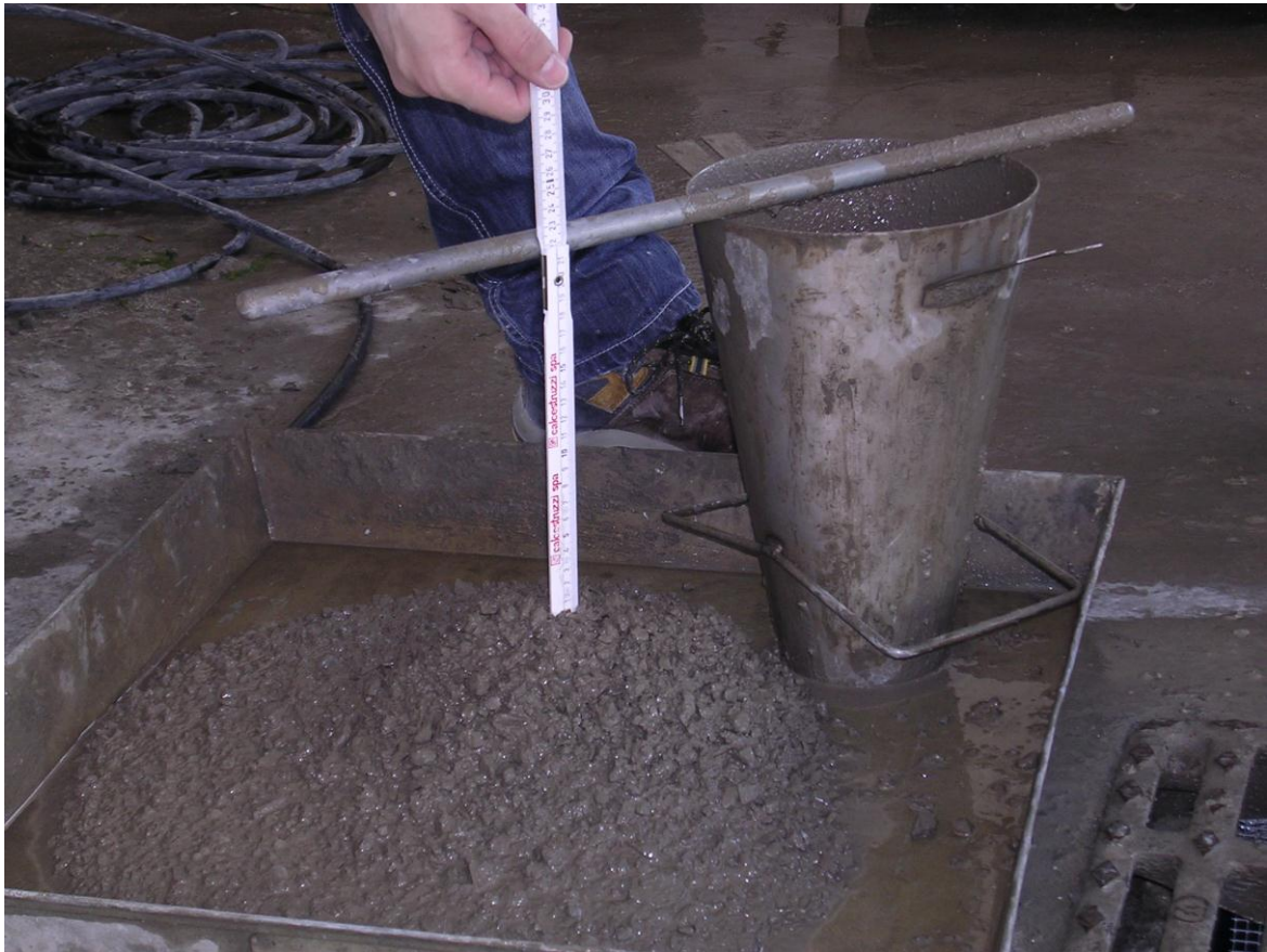
Fig. 7 - Slump 100% coarse and fine recycled aggregates, 5' - 1RC
