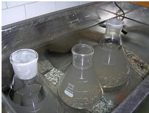
Fig. 8 – Pycnometers with natural and recycled aggregates in thermostatic bath
