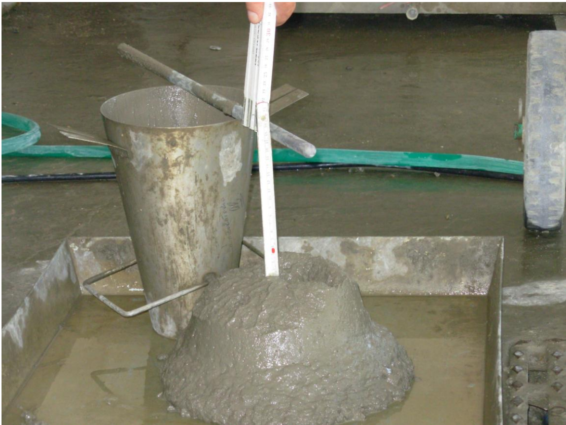
Fig. 10 - Slump 100% coarse recycled aggregates, fine totally natural , 30' - 5RC
