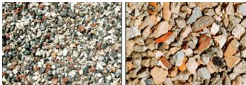
Fig. 2 – Fine and coarse recycled aggregate derived from demolition waste
