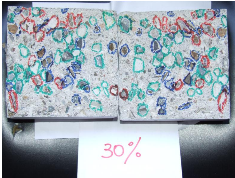
Fig. 37 - Specimen after-tensile test, 30% of coarse recycled aggregates
