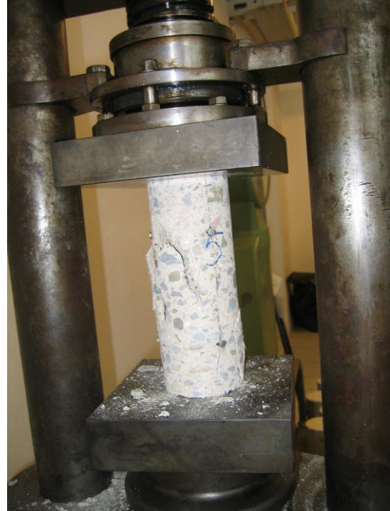
Fig. 25 - Compressive test on specimen made with 50% of coarse and fine recycled aggregates + 50% naturals
