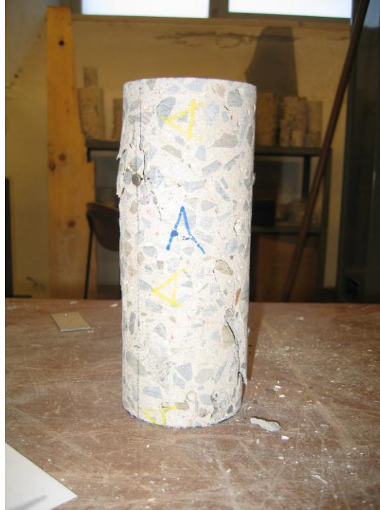
Fig. 27 - Compressive test on specimen of normal concrete
