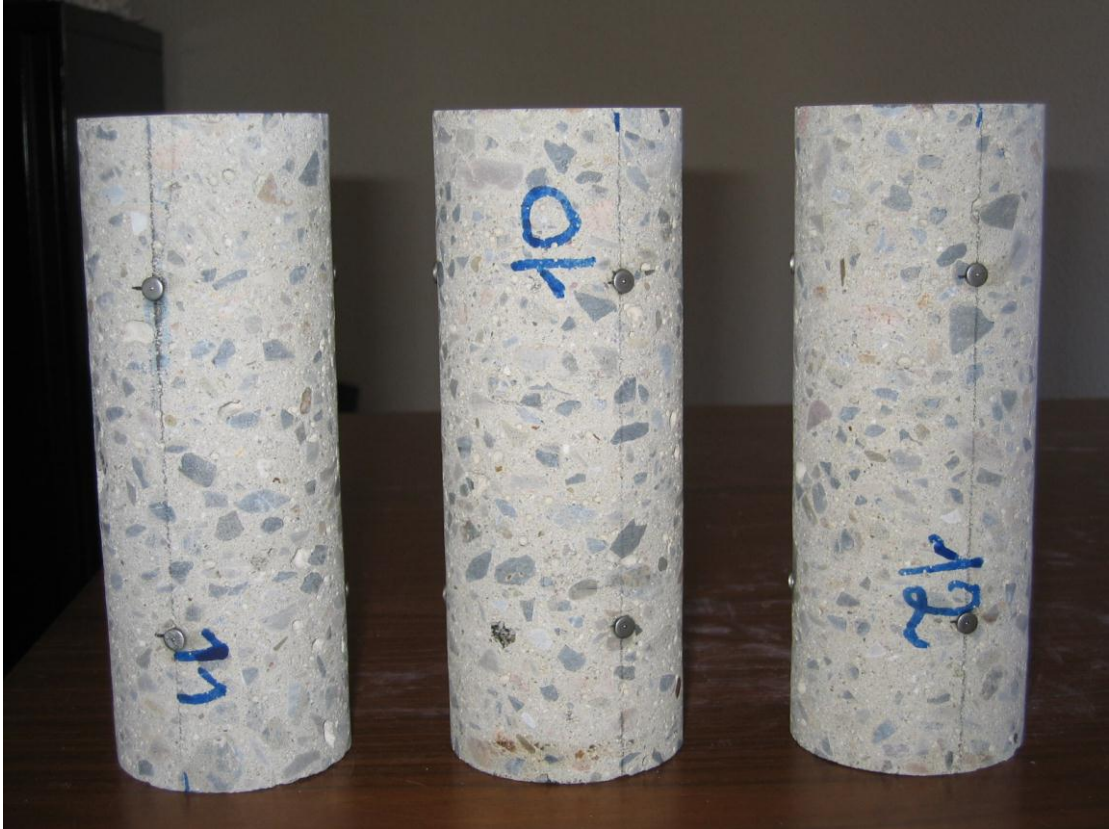
Fig. 41 - Cylinder specimens made with 100% of coarse recycled aggregates
