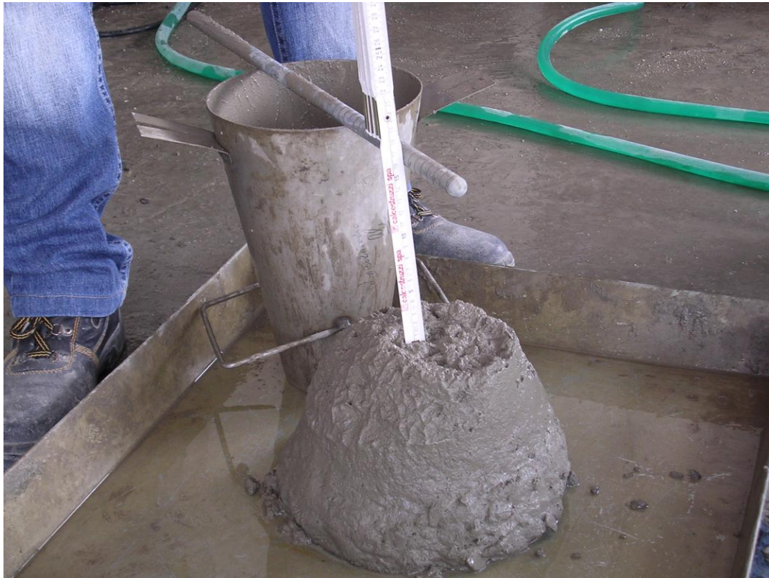
Fig. 13 - Slump conventional concrete, 5 °
