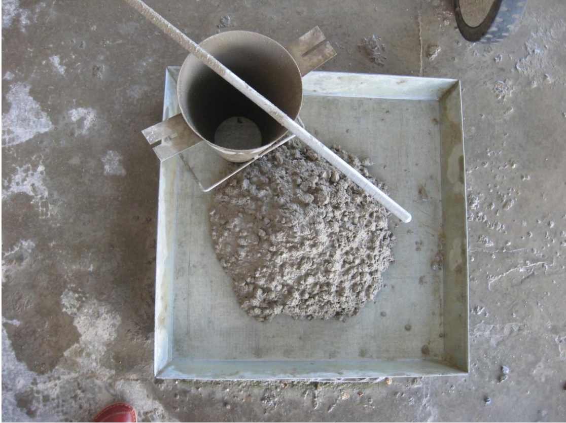
Fig. 11 - Slump 100% coarse recycled aggregates, fine totally natural , 5' – 9RC
