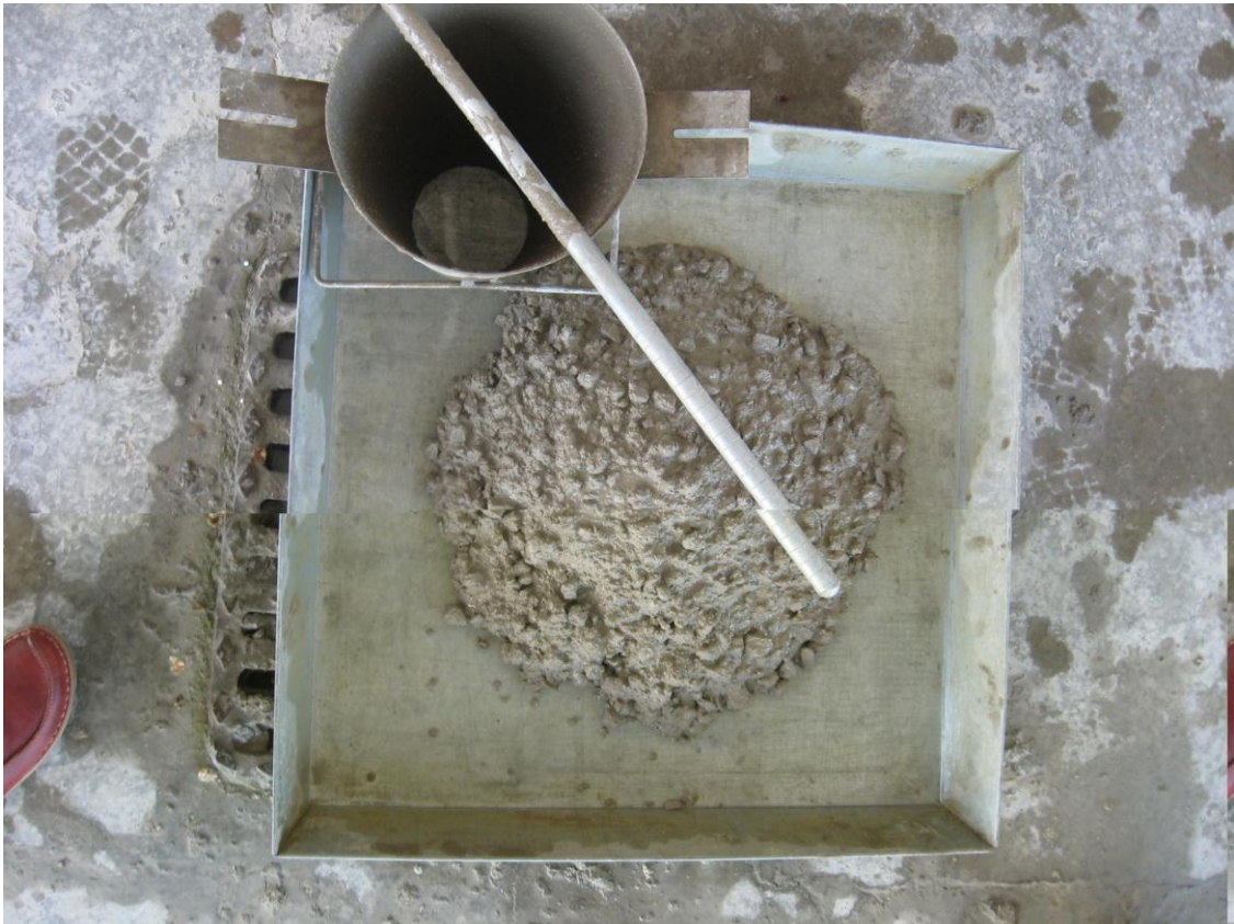
Fig. 12 - Slump 100% coarse recycled aggregates, fine totally natural, 30' - 9RC
