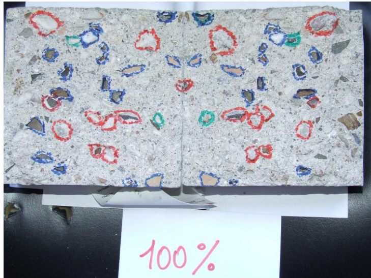
Fig. 34 - Specimen after tensile test, 100% of coarse recycled aggregates
