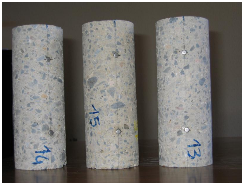
Fig. 38 - Cylinder specimens made with 100% of coarse and fine recycled aggregates
