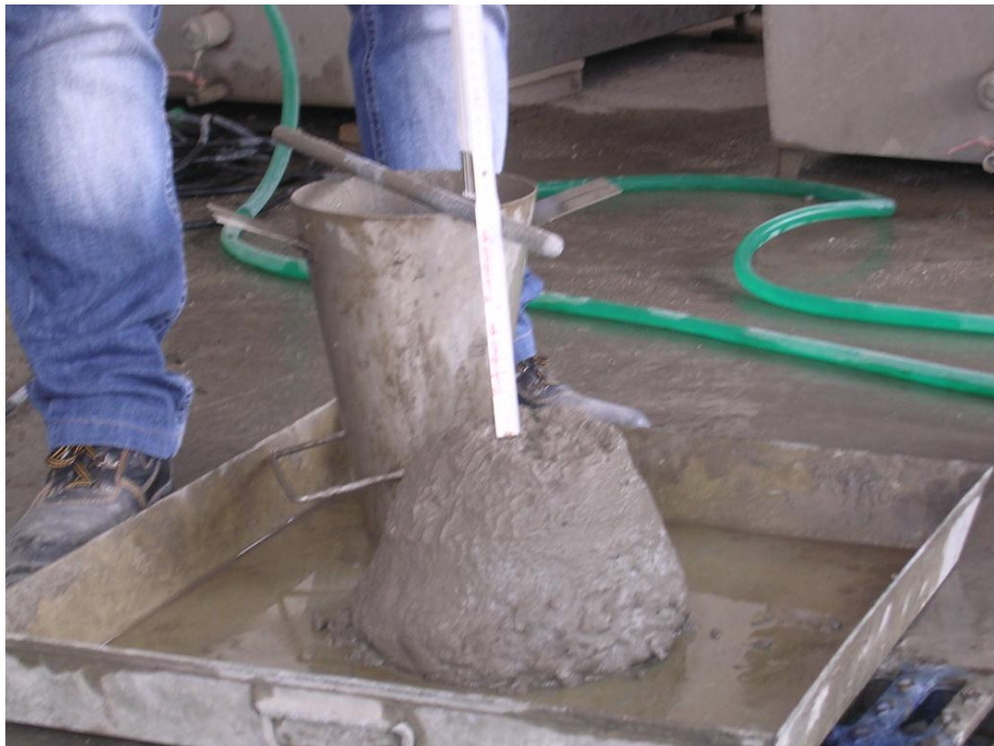
Fig. 14 - Slump conventional concrete, 30 °
