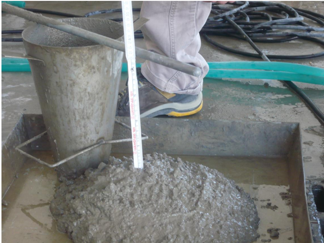
Fig. 3 - Slump 50% coarse and fine recycled aggregate + 50% coarse and fine natural aggregates, 5' - 3RC
