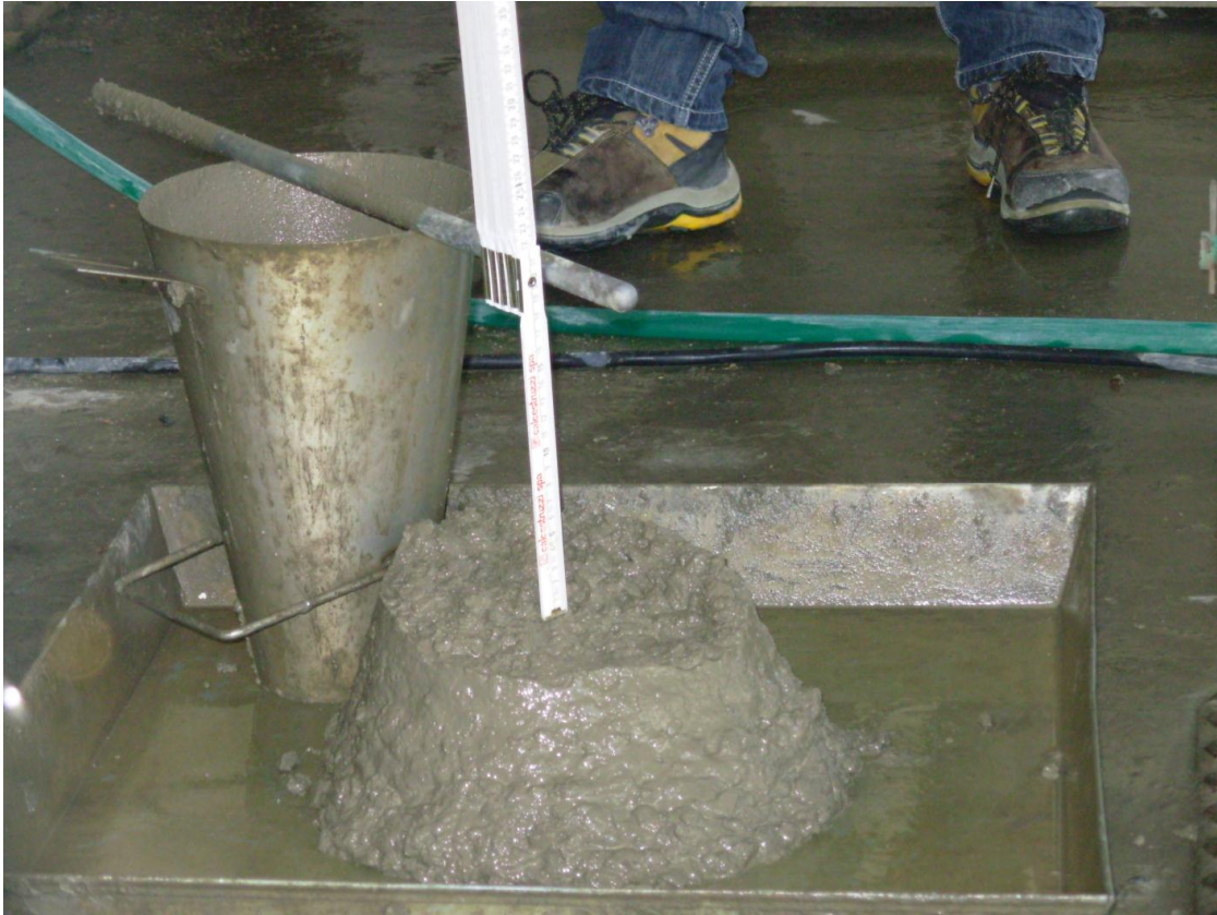
Fig. 6 - Slump 20% coarse and fine recycled aggregates + 80% coarse and fine natural aggregates, 30' - 4RC
