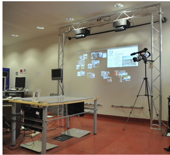
Figure 7.1: The interactive space: notice the multitouch table and the wall sized interactive displays; camera are arranged in the space for capturing the activities for research purposes
