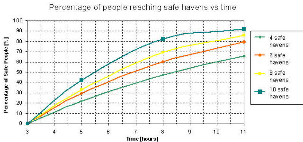
Figure 14.2: The effects of the number of safe havens on the percentage of people reaching safety
