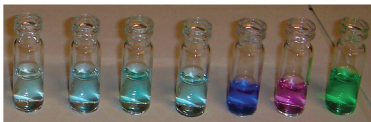
Figure 1.13. Colour change of 51 (10 -3 M) after addition of different anions in CH 3 CN. From left to right: free receptor; +1 eq. F - ; +1 eq. Cl - ; +1 eq. Br - ; +1 eq. CN - ; +2 eq. CN - ; +1 eq. I - .
