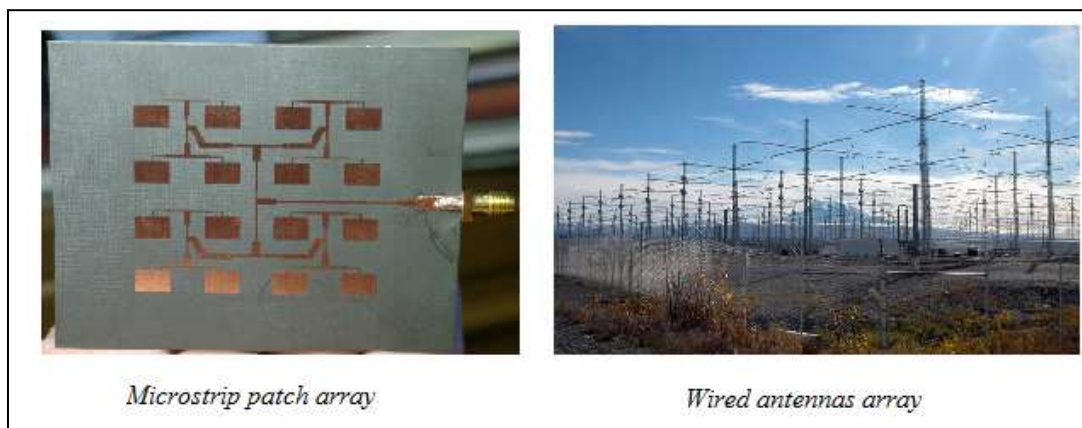
Figure 2.8. Example of array antennas
