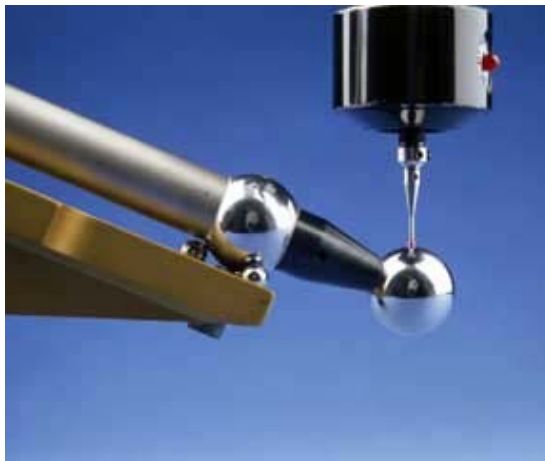
Fig. 2.11. Ball Bar with probe
