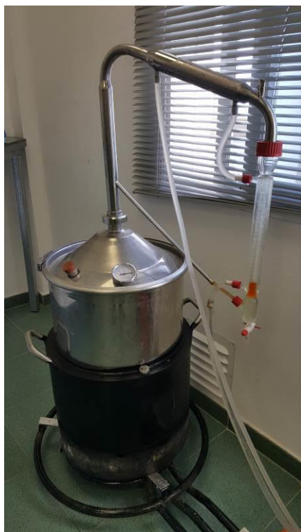
Figure 22: Extraction of essential oil from different S. montana plots at laboratory pilot plant-scale.
