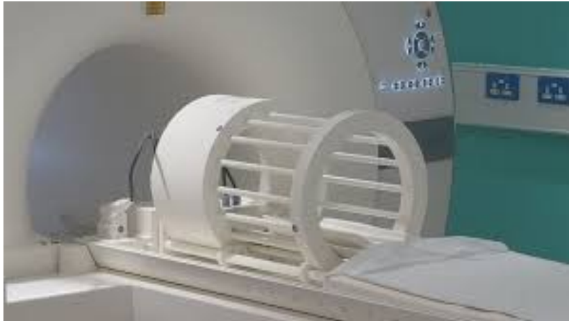
Figure 4.1 An example of birdcage coil for MRI
