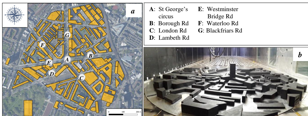
Figure 4.7 - Panel a: Plan view of the MAGIC site in London. The ortho-photo view is overlapped with the 150 model buildings. Panel b: MAGIC model with flat roofs, created for experiments; wind tunnel view on the rotating turntable.
