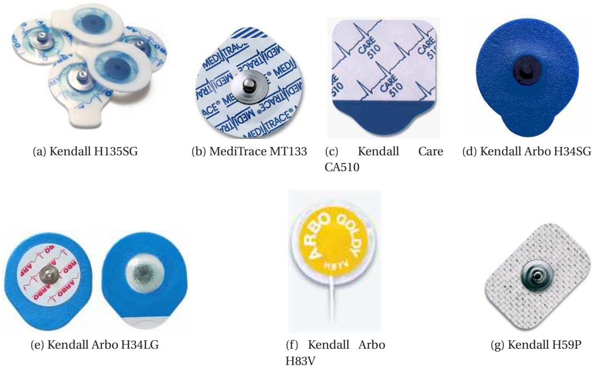
Figure 3.7: Tested disposable commercial electrodes
