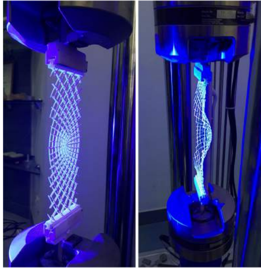
Fig. 22 Bias extension test on parabolic pantographic fabric. Out-of-plane buckling is observed after critical loading
