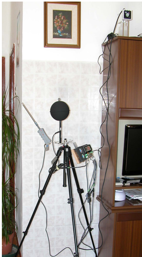
Figure 2. Full microclimatic station for the measurement of environmental parameters affecting occupants' global comfort sensation, according to ISO 7726 [7].
