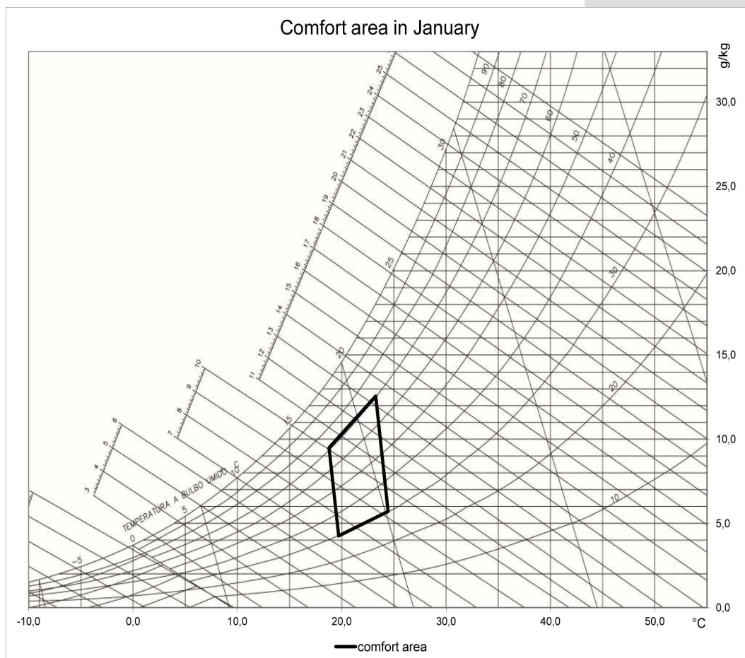
Figure 5. Comfort area drawn for winter conditions in an office space. MET=1,2 ; CLO=1 ; v_a=0,1 m/s; MRT=t_a ; PMV_{II}=-0,5 ; PMV_{III}=0,5 (space category B).
