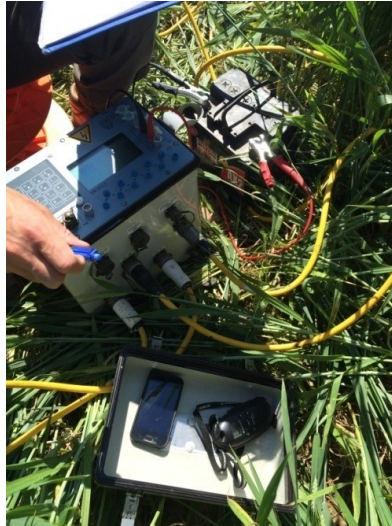
Figure 4.45: Syscal Pro georesistivity meter by IRIS Instruments.
