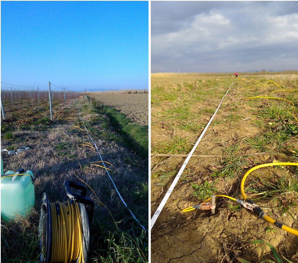
Figure 4.48: First figure on the left represents electrical cables for the El04 line. The relative metric cable is visible in white, useful for establishing the electrodes spacing at a distance of 2 meters. Second image on the right shows the detail of the electrode into the ground during the acquisition of the El05 line.
