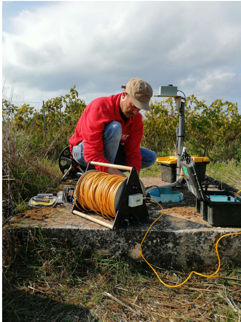
Figure 4.1: Site investigation for Regional Monitoring well P.10745 located in the municipal area of Castagneto Carducci. The instrumentation used for field investigations consists of: interface probe for water table level measurements, weight for well depth measuring, interface probe for measuring electrical conductivity, video underwater camera for inspection of the well.
