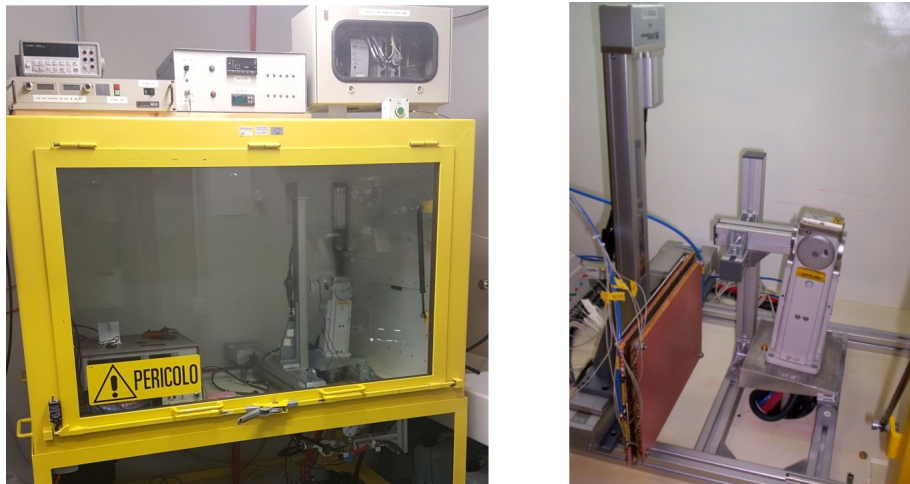
FIGURE 3.32. Left: the safety shielded enclosure with the X-Ray tube and the moving system inside. Right: picture of the X-Ray tube and the moving system.
