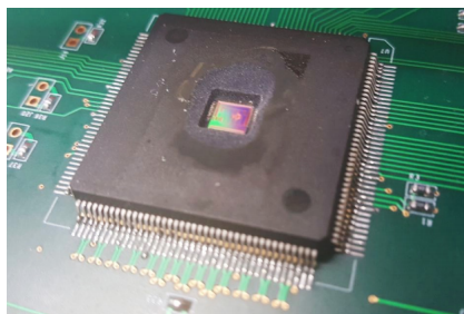
FIGURE 3.33. Picture of the nSYNC package and the exposed die after the decapsulation.
