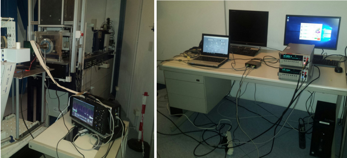
FIGURE 3.21. Left: picture of the final experimental setup within the CATANA room, in particular the nSYNC test board and the oscilloscope are shown. Right: The main control PC, the two power supplies and the various connections are shown.
