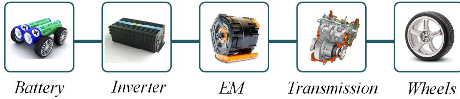
Figure I.1 – Schematic representation of an electric propulsion system.
