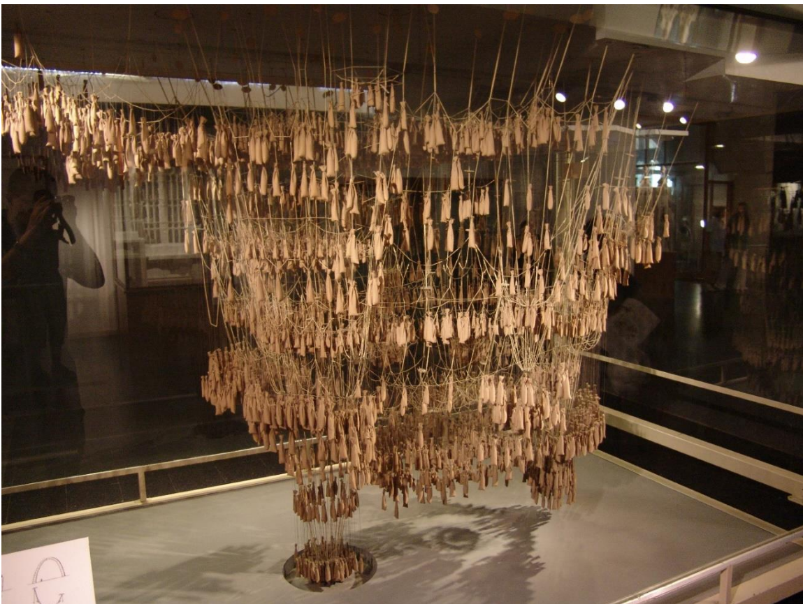
Figure 1. 1 Physical inverted model for the Church of Colònia Güell built up by Antonio Gaudí
