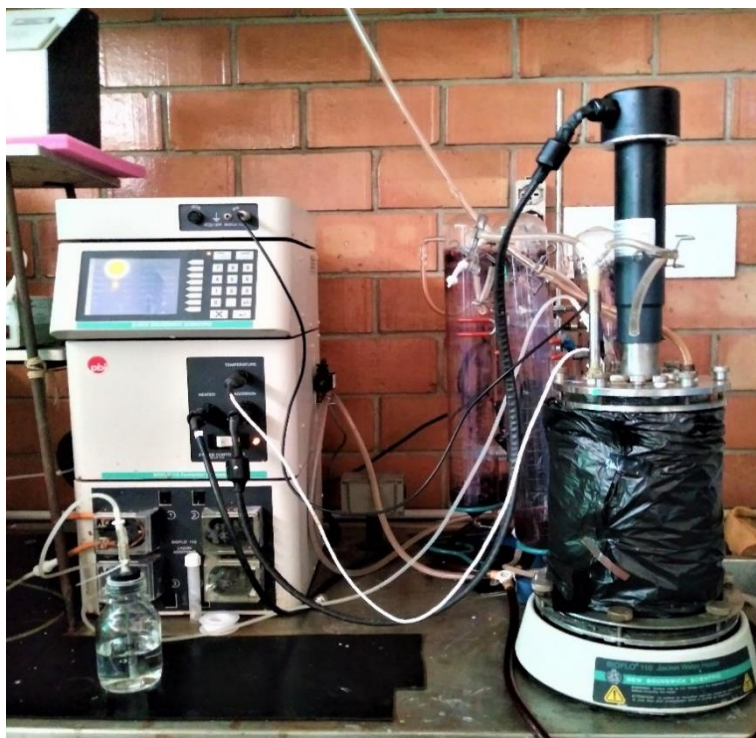
Figure 6.2: BIOFLO 110 reactor for dark fermentation (New Brunswick Scientific; Bio Command Lite software).
