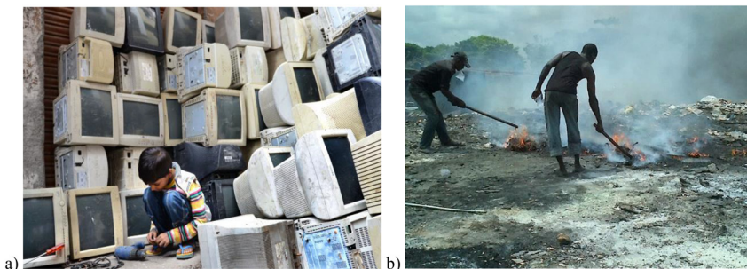
Fig. 4: Activities associated with informal e-waste recycling – (a) manual dismantling (source: D. Chatterjee); (b) open burning of e-waste to recover valuable materials (Source: O. E. Popoola).
