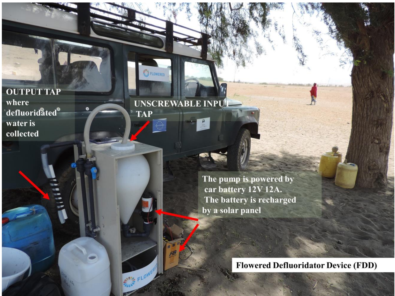
Figure S3. Configuration of the Flowered Defluorinator Device (FDD)
