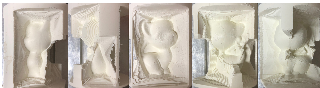
Figure A.21: Finishing phase. Side regions finished with a 1mm ball cutter.
