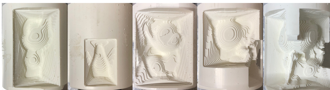
Figure A.20: Roughing phase. Side regions finished with a 3mm flat cutter.
