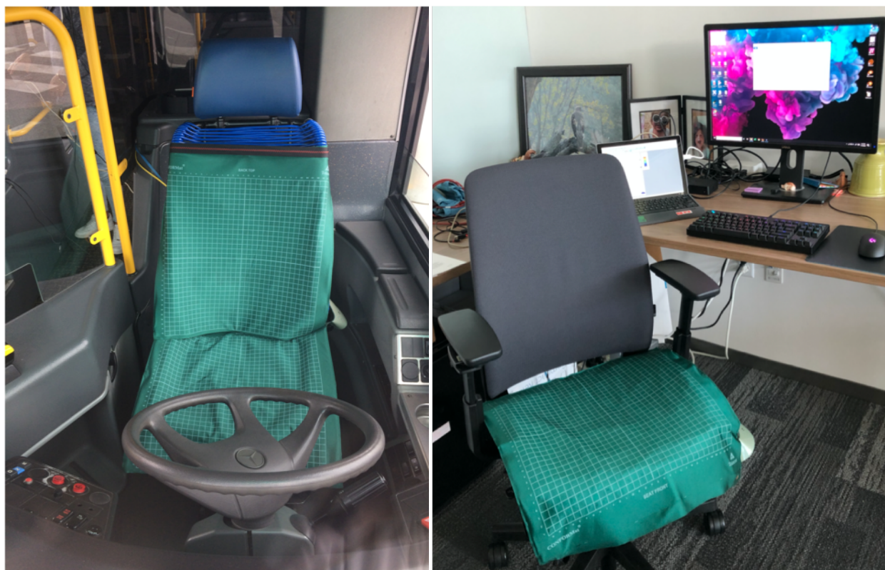
Figure 6. 1: An example of the workstations equipped with the pressure sensitive mat system. On the left the bus cockpit, on the right the office workers' desk.
