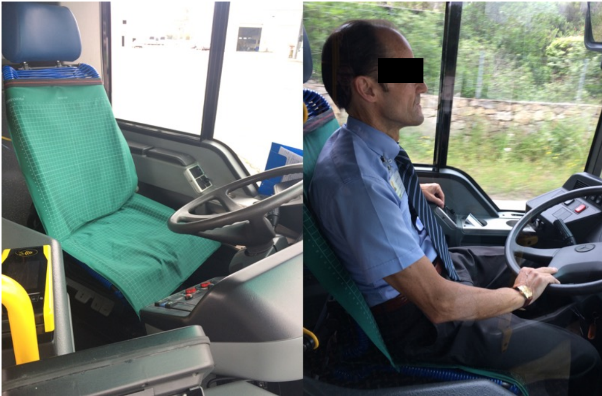
Figure 8.1: Photo of the pressure sensitive mats positioned on the seat (left). Bus driver during a driving session (right).
