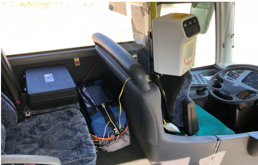
Figure 9.1: Photo of the pressure sensitive mats positioned on the seat and connected to the computer.
