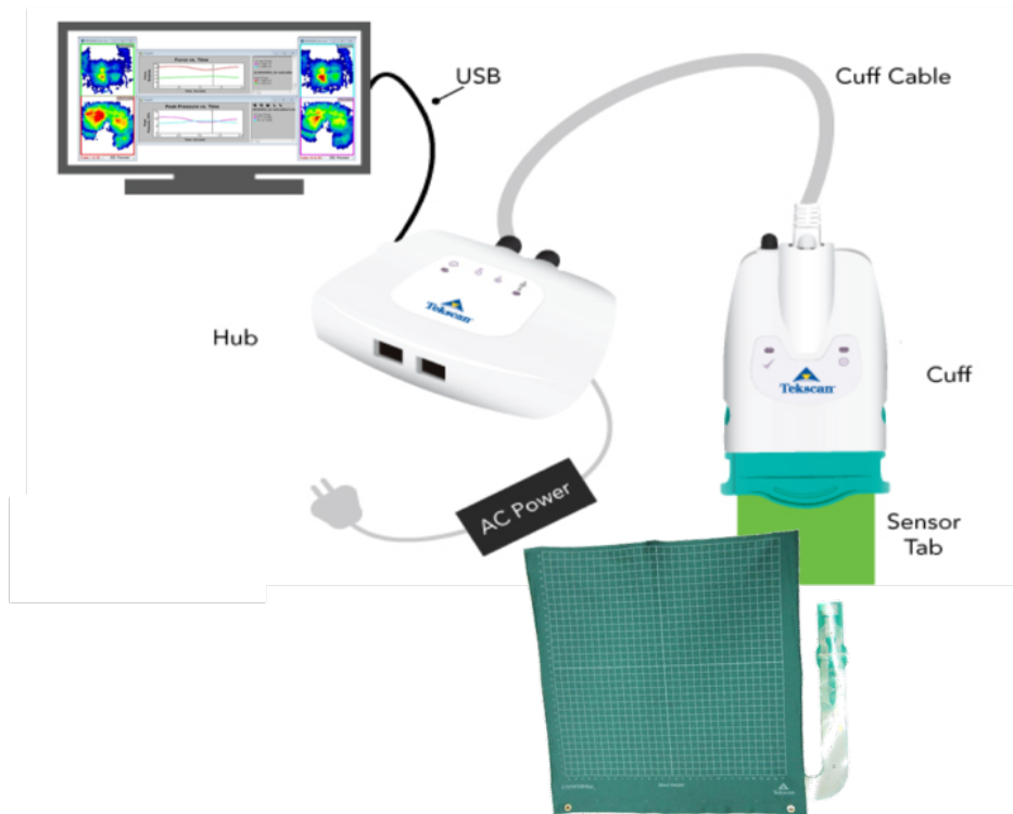
Figure 5.8: Schematic representation of the Tekscan external scanning electronics connected to the PC and to the sensing unit
