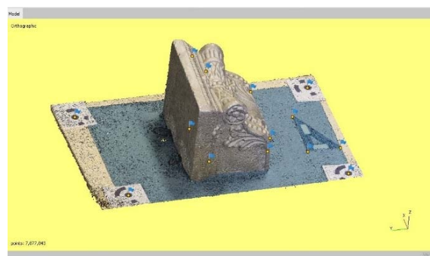
Fig. 17: Cast of modillion - “Building dense point cloud”
