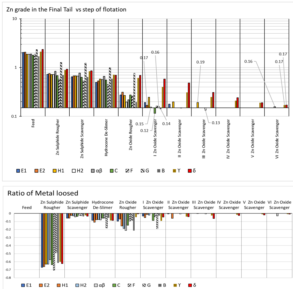
Figure 5.7 Histograms of Zn concentrations and metal units in final waste for 11 test groups
