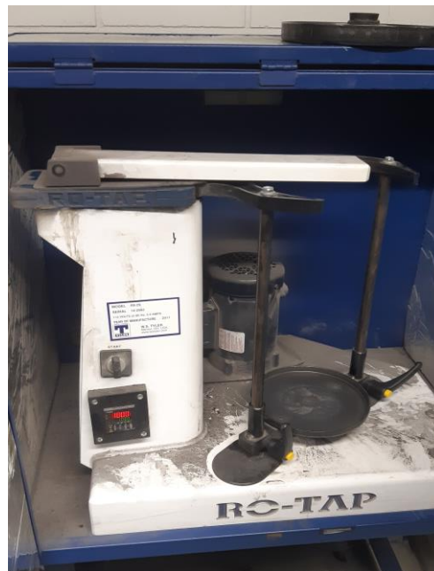
Figure 3.13 Ro-Tap sieve shaker, model RX-29
