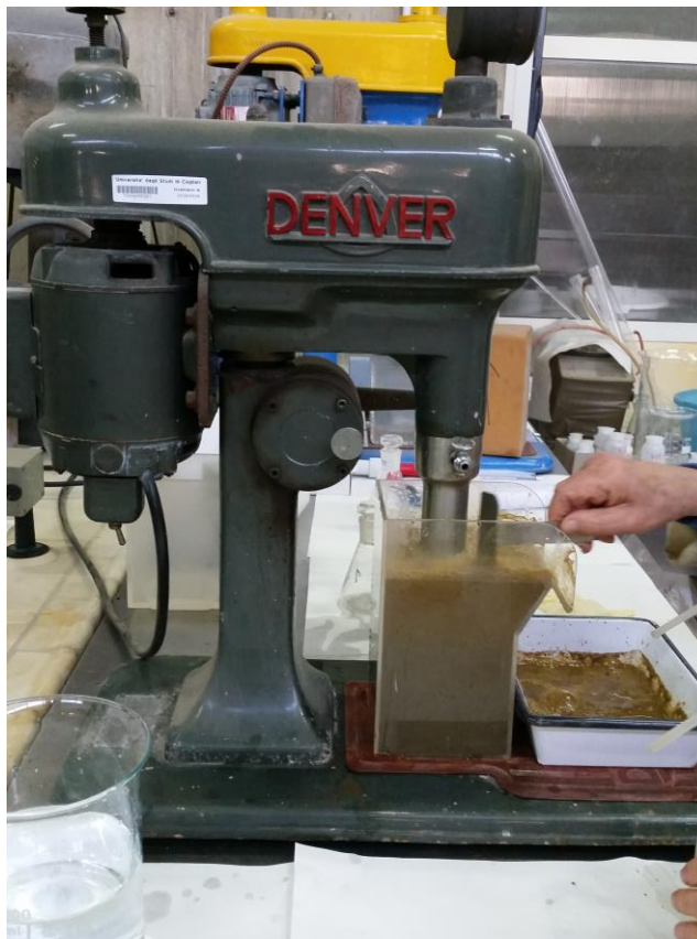
Figure 3.3 Denver flotation machine
