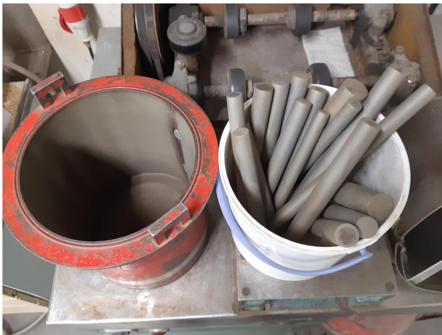
Figure 3.12 Mild steel laboratory rod mill
