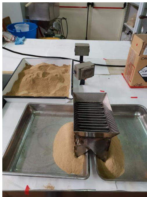
Figure 3.10 Quartering with Jones divider.
