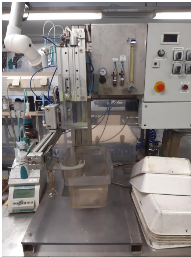
Figure 3.4 "GTK" Flotation machine (Outokumpu type)
