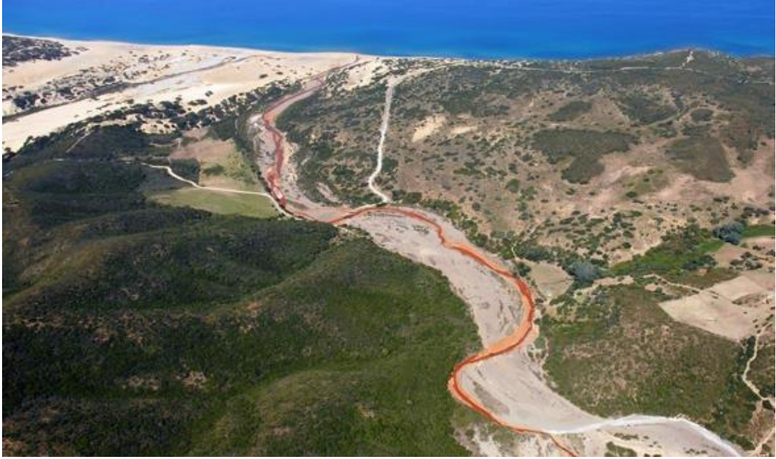
Figure 1.2 Contamination of Rio Piscinas (south-western coast of Sardinia), caused by the transport of mining residues [6].
