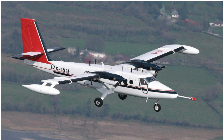
Figure 2-5 De Havilland Twin Otter survey aircraft. The wingtips contain the electromagnetic transmitter and receiver coils and one magnetometer sensor (taken from (Hodgson & Young, 2016)).
