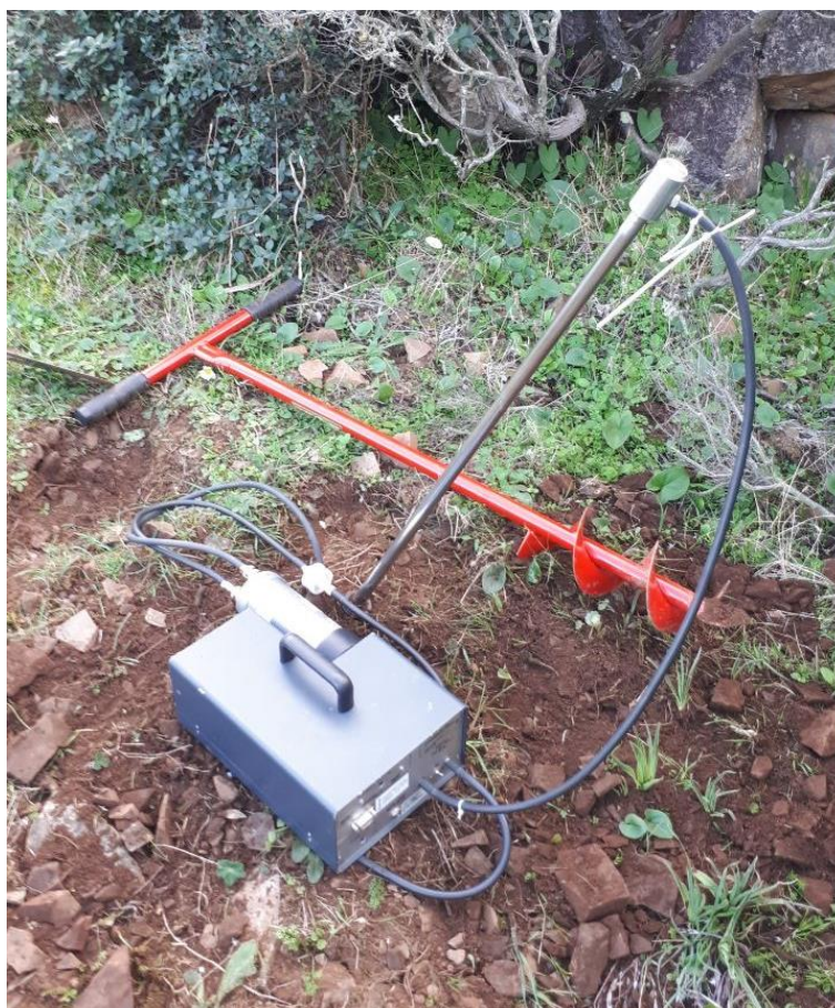
Figure 8-7: Active soil gas radon measurement with an MR-1 instrument
