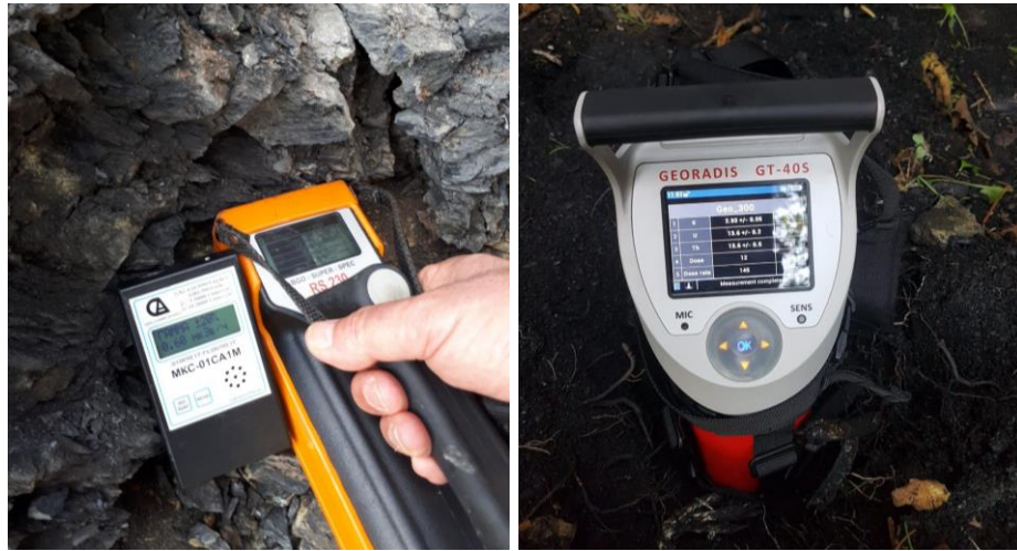
Figure 2-4: Application of RS-230 (left) and GT-40S (right) spectrometers for field surveying of naturally occurring radioactive elements
