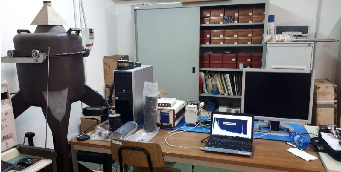
Figure 2-1: NaI (TI) gamma spectrometer of the nuclear physics laboratory of the University of Cagliari.
