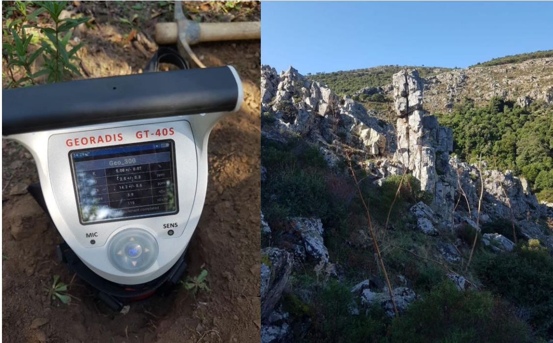
Figure 8-4: natural activity detection at the test point location (left) and the rocks belonging to the Punta Serpeddi Formation (right).
