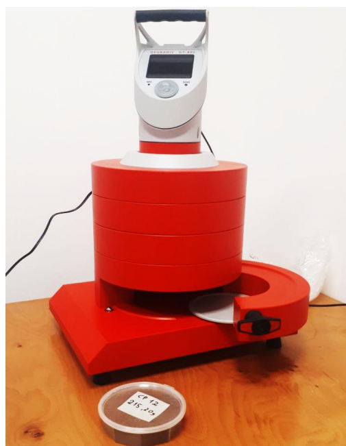
Figure 8-9: The GT-40S gamma-ray spectrometer incorporated into the Pb shielding collimator and a sample prepared for testing.
