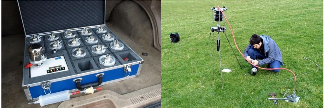
Figure 2-9: Instruments for sampling the soil air and in-situ detection of soil gas radon.
