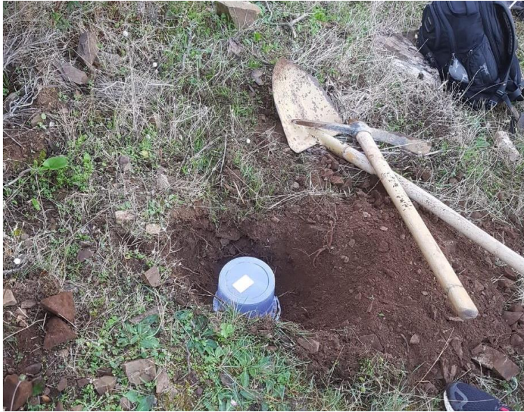
Figure 8-6: Installation of the passive radon detector can
