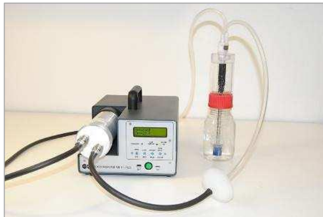
Figure 2-10: Setup for radon in water measurements using MR1 radon detector and ACQUAKIT accessory (Cardellini, 2017)
