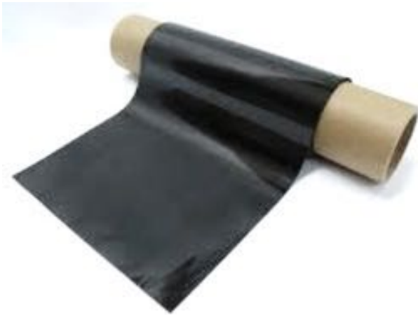
Figure 4.3 – Pre-preg plies (carbon - epoxy).
