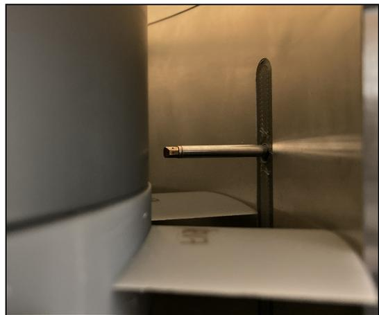
(c) Aerodynamic probe in the Wells turbine.
