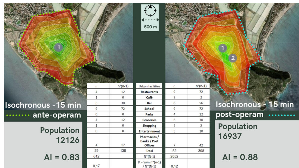
Figure 5. Isochrone (intervals 2 min) 15 min by foot (ante and post operam) and relative AI (attractiveness index). Author: Balletto G. and Milesi A. (2021). Source: https://maps.openrouteservice.org and https://www.walkscore.com , last accessed 1 October 2021.
