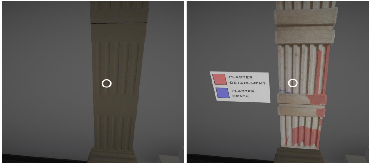
Figure 10. An example of an interaction providing information about a simple decay state analysis. On the left the model before the interaction, on the right the decay analysis overlaid on the model after the interaction.
