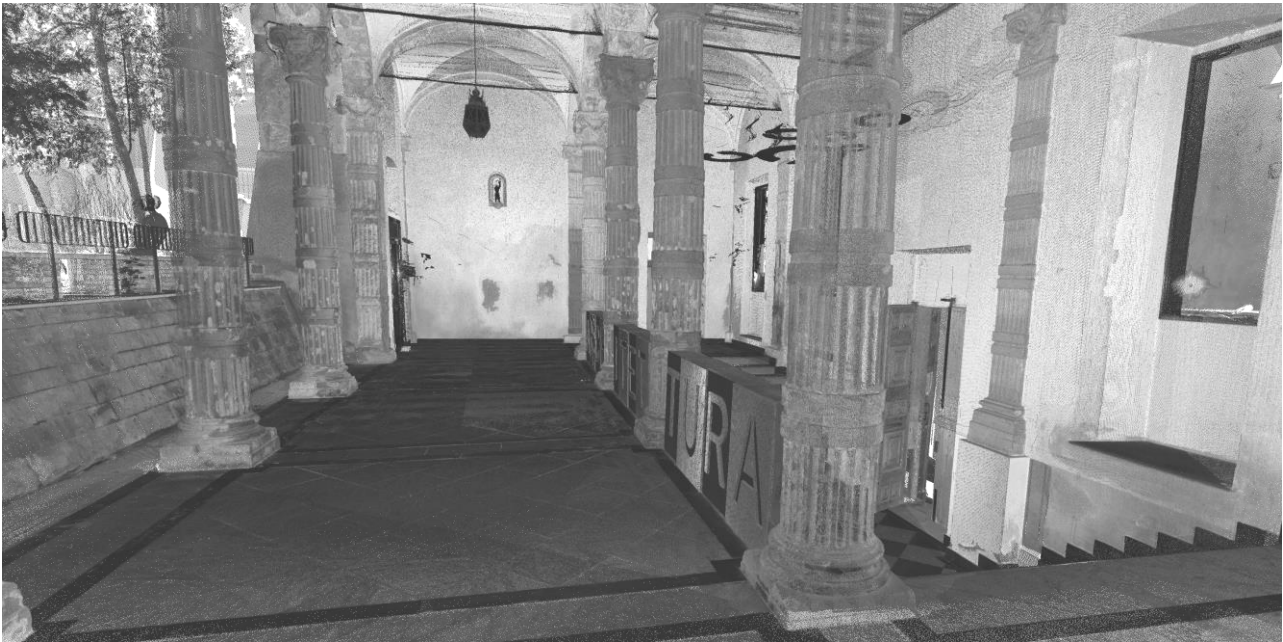
Figure 6. An image of the registered point cloud of the atrium.
