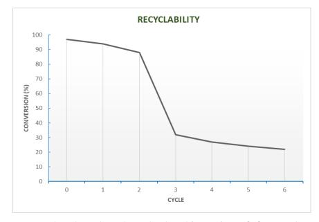
**Figure 4.** Pd-wool complex cycle trend. Adapted from Reference [34]. Copyright 2012, Royal Society of Chemistry.
