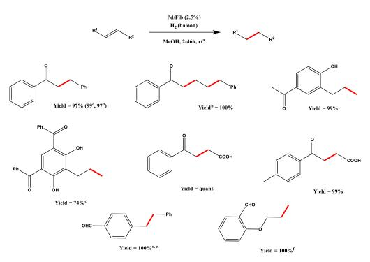
**Scheme 4.** Olefins' reduction scope, all hydrogenations were performed using 2.5% Pd/Fib; <sup>a</sup> Unless otherwise specified, reactions were performed in 5 mL of MeOH under ambient hydrogen pressure at r.t.; <sup>b</sup> Yields after purification; <sup>c</sup> H<sub>2</sub> pressure of 5 atm; <sup>d</sup> Reaction performed at 50 °C; <sup>e</sup> solvent = 5 mL CH<sub>2</sub>Cl<sub>2</sub>; <sup>f</sup> solvent = 5 mL AcOEt. Adapted from Reference [66]. Copyright 2005, Elsevier.
