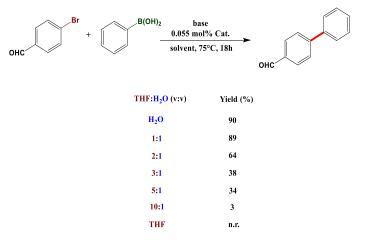
**Figure 5.** Progressive solvent scale for the reaction. Adapted from Reference [34]. Copyright 2012, Royal Society of Chemistry.
