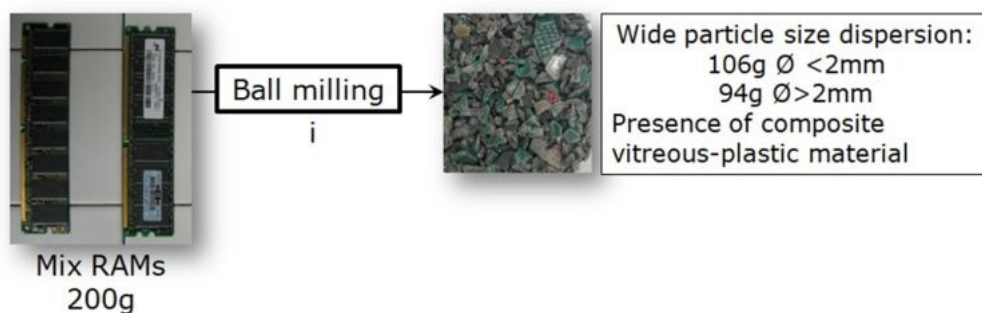
Figure 5. Preparation of the RAM #R#G#M sample. i = 24\text{h} , room temperature; stainless steel jar planetary apparatus: 4-stages mill, 300 rpm; hardmetal balls \varnothing = 6 mm, weight = 1.4 Kg; solvent: Carbsyn, 250 mL.
