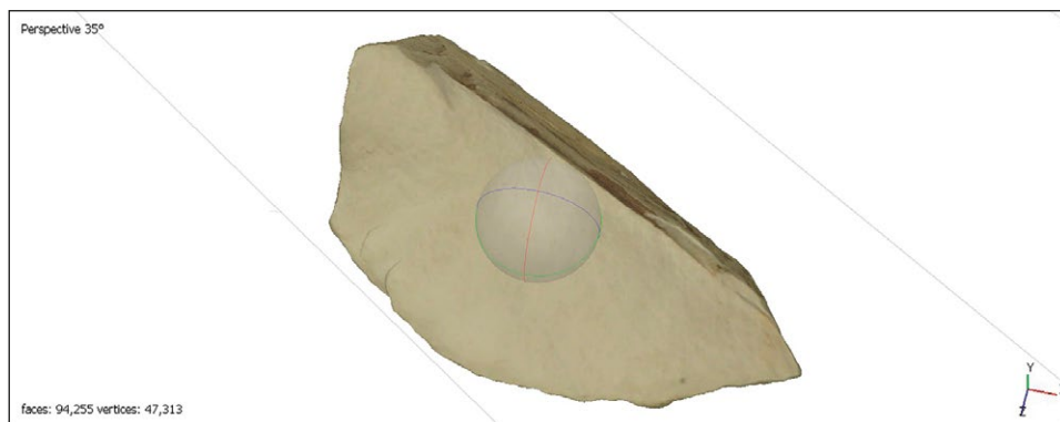
Fig. 4 – Texture model of the selected limestone block. The lack of transparent and reflecting surfaces and a simple geometric shape allowed for an easy processing of the 3D model.
