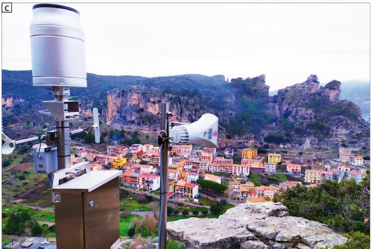
Figure 45 –A) Conceptual model of the work. B) Alarm levels. C) Monitoring station 1 whit weather station the siren.
