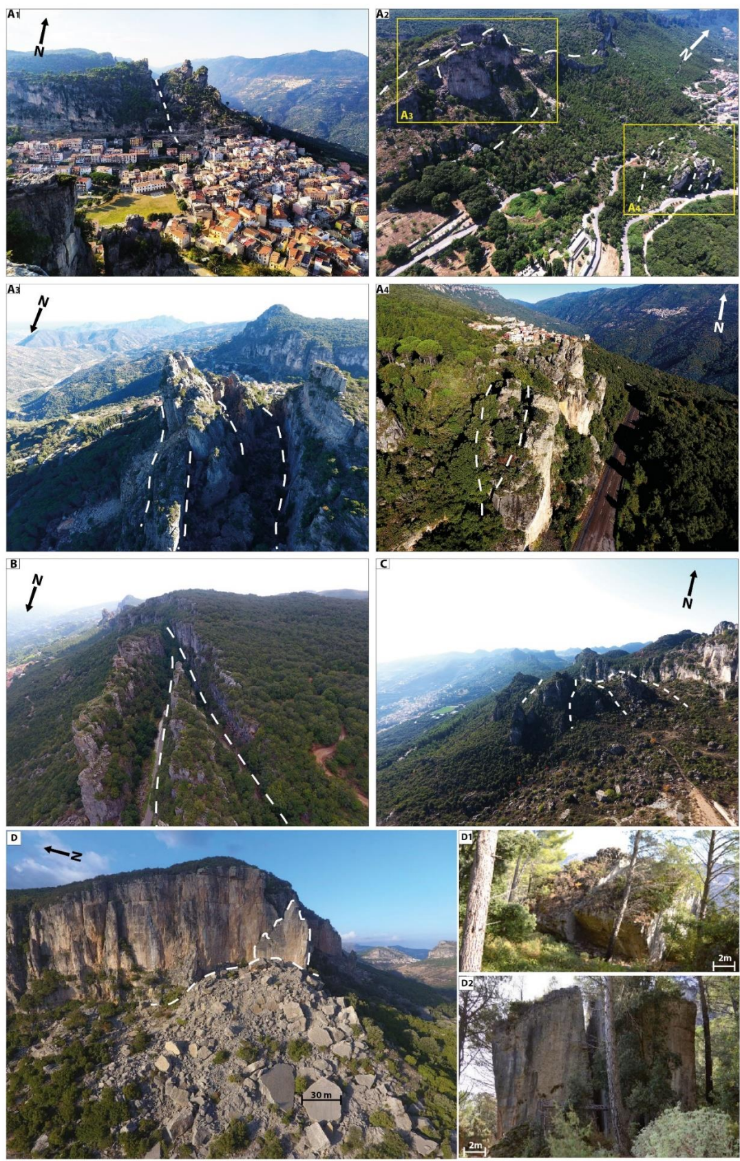
Figure 18 UAV images of the DGSD showing the major geomorphological and structural features. The white dashed lines represent the major extensional trenches. (A1). Panoramic view of the Ulassai Village. (A2) Bruncu Pranedda DGSD. (A3) Top slope sector. (A4) Middle slope sector. (B) San Giorgio DGSD. (C) Tisiddu Mountain DGSD. (D) Evidence of collapse deposits of rock avalanches. Recent collapse near Ulassai Village. (D1, D2) Palaeo-collapses of mega-blocks, 20–40 m for each side.
