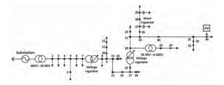
Figure 2: Test system: IEEE 34 Node Test feeder
