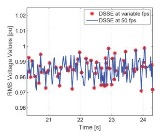
Figure 3: Case 3: voltage magnitude estimation at node 25 with fixed and variable rate DSSE.
