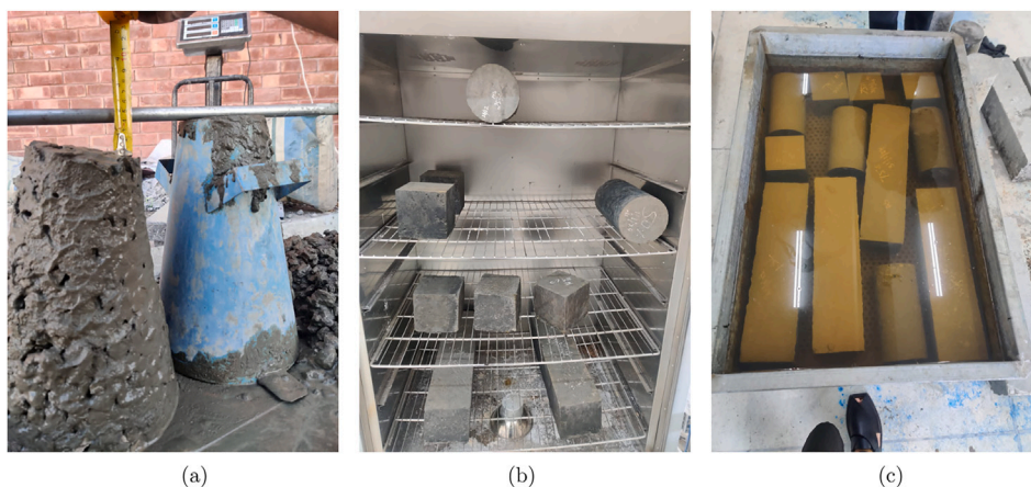
Fig. 4. Preparation and conditioning of concrete specimens: (a) measurement of slump to assess fresh concrete workability; (b) oven-drying of cubes and cylinders prior to testing; (c) 28-day water curing of beams and cylinders in a controlled tank.
