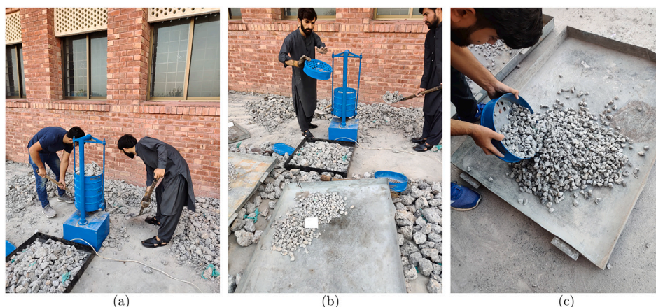
Fig. 3. Sieve analysis of RCA: (a) loading the crushed material into the sieve stack; (b) manual agitation and intermediate separation of aggregate fractions; (c) collection of the sieved RCA retained on the target sieve size.
