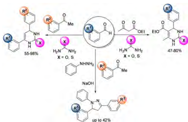
Scheme 30. Multicomponent reactions for the synthesis of dihydropyrimidinones, dihydropyrimidinethiones, and pyrazolines under mechanical activation. Adapted with permission from Ref. [160]. Copyright 2020, the authors.
