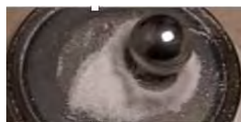
Figure 4. A frame of the impact between ball and jar wall.
