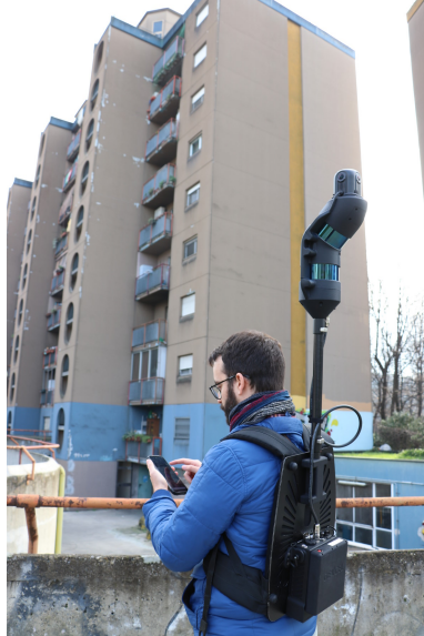
Figure 5.5: Starting the acquisition with the mobile mapping prototype in Milan. The capturing system is controlled by a PDA connected via WIFI with the SoC.
