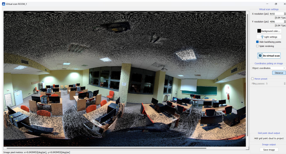
Figure 5.21: The virtual scan process maps each pixel of the 8K image onto the coordinate system of the mobile point cloud.
