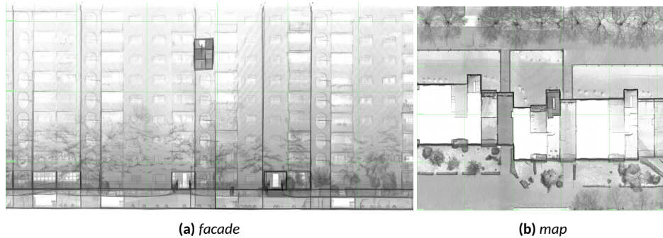
Figure 5.8: Blueprint and facade view extracted from the mobile mapping of the MM building in Milan.
