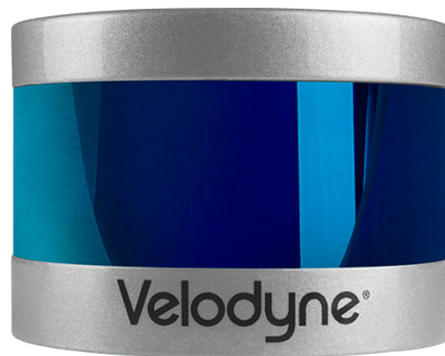
Figure 2.4: Velodyne [4] VLP-16 rotative LiDAR sensor
