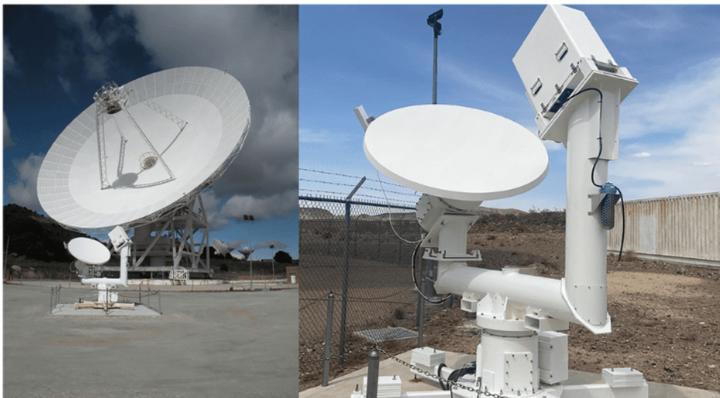
Figure 4.5: Advanced Water Vapor Radiometer units next to the DSN 34-meter antennas (Buccino et al. 2021).
