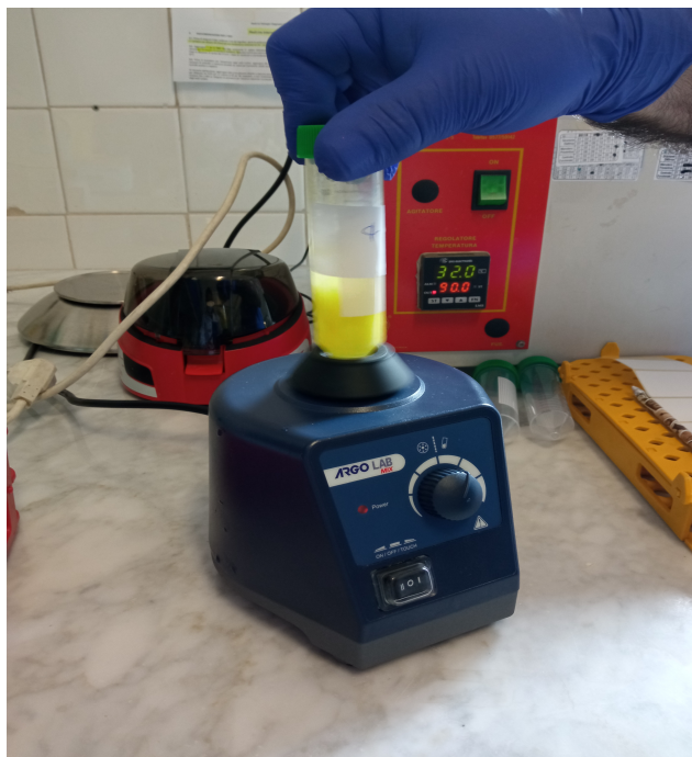
Figure 3. EVOO vortexed with 3% of Hydrogen Peroxide as a catalyst of ROS production.
