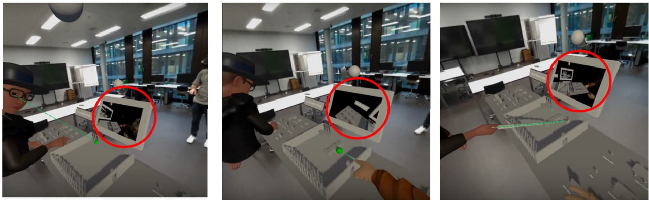
Figure P 66. Three pointer styles (green ball indicates the position of the "pointer"). Left: Gaze pointer visualizes where the gaze hits the scene. Middle: Finger pointer extends the finger with a semi-transparent line, enabling a natural pointing behavior with an extended finger. Right: A representation of a physical pointer, similar the one presented by Brägger et al., 2022. One of the shared view concepts, i.e., picture-in-picture view is highlighted with a red circle in all three panels.
