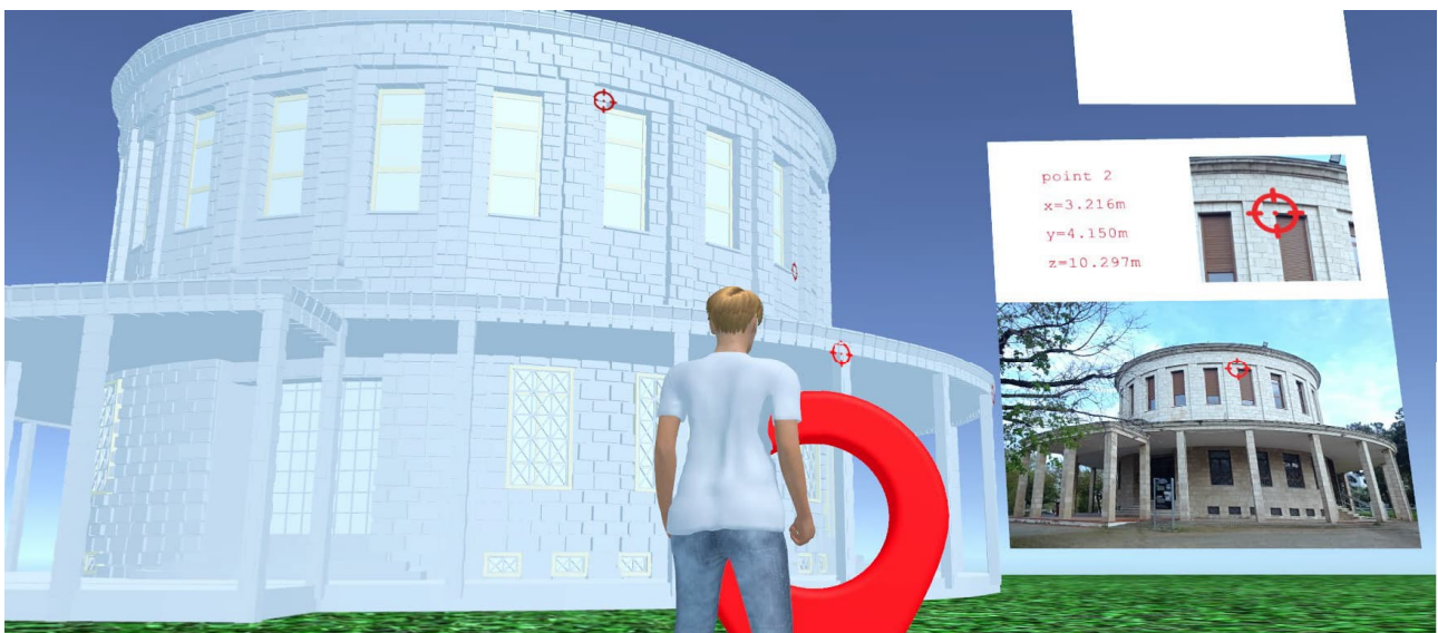
Figure 25. The 3D representation of the observatory, the student (as an avatar), the predefined points (big 3D red pointers) to capture images and the Ground Control Points (GCPs) on the surface of the observatory.
