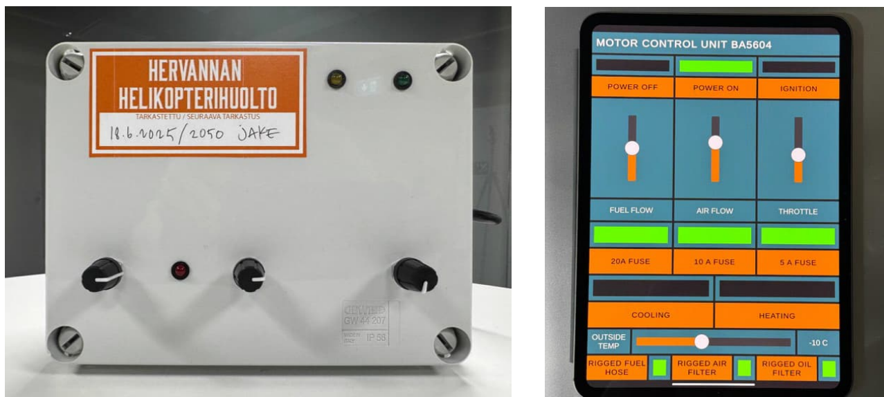
Figure 31. The input devices for the MQTT broker. The physical “IoT box” includes three rotary-encoded dials to handle fuel flow, air flow, and throttle. A red LED turns on or blinks when AFR goes slightly out of range or it reaches critical levels. The iPad application emulated the box, with the three sliders on the upper part of the UI.
