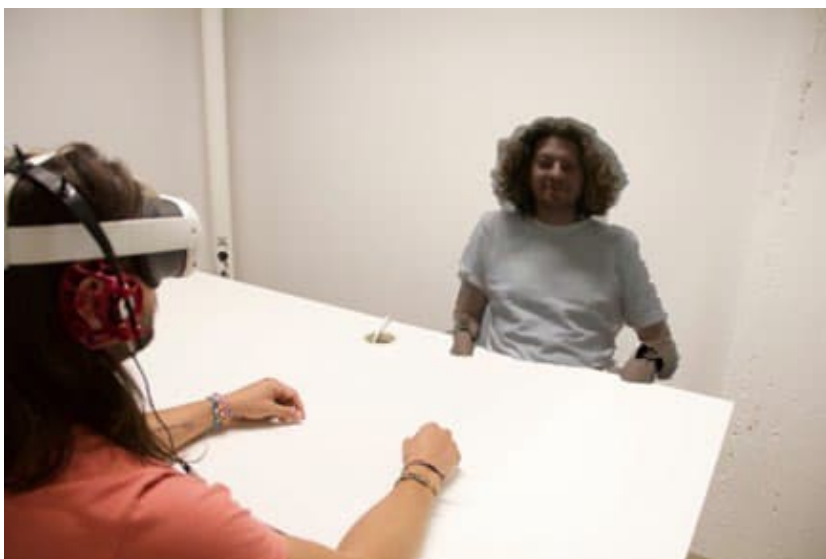
Figure P 37. Holographic calling setup with HMD and transparent headphones.
