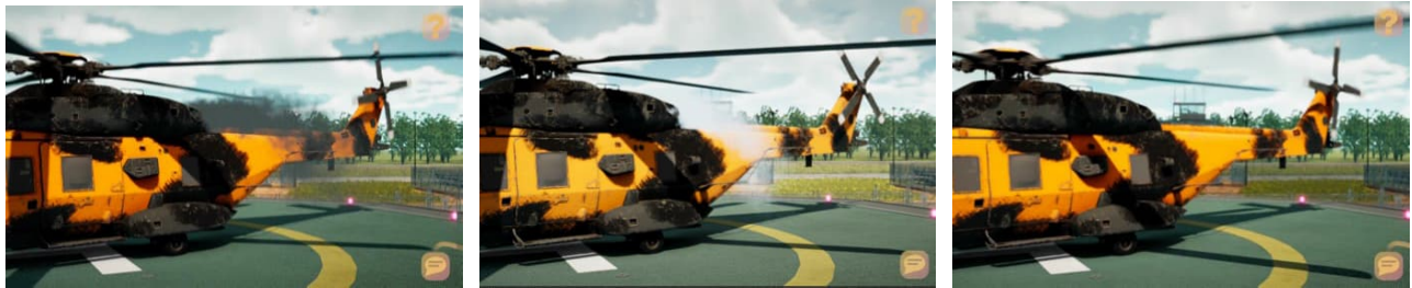
Figure 30. The visual effects coming from the helicopter model. Black smoke (on the left) indicates a “rich” condition, where too much fuel is present on the mixture, while white/grey smoke indicate a “lean” condition (on the center) with excessive air flow. Different engine sounds are also played for different conditions.
