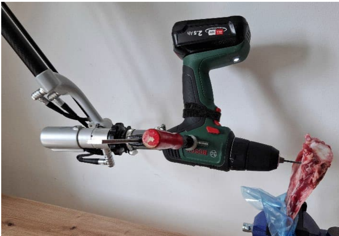
Figure 12. Recording of the drilling progression speed with a Virtuose 6D High-Force device.
