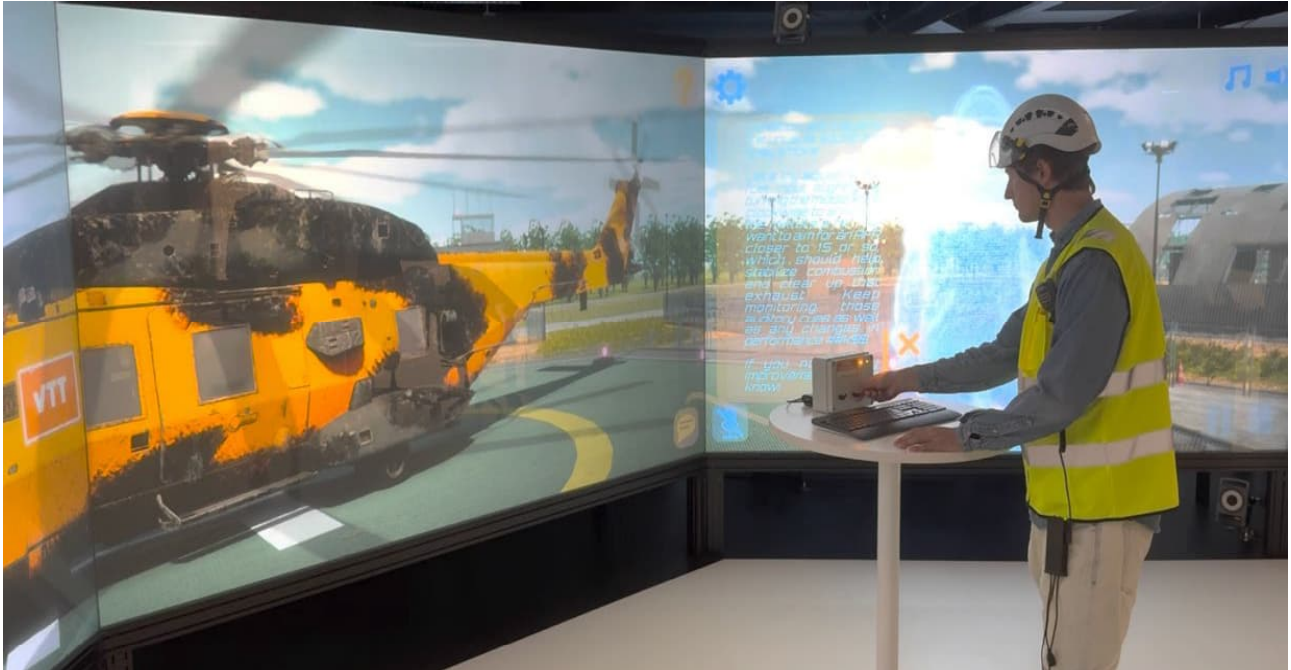
Figure 28. Overview of the simulator setup. It includes a wall-sized display, a push-to-talk microphone, and an “IoT box” with 3 rotating dials and a red LED light. Keyboard and mouse are used to customize the UI.
