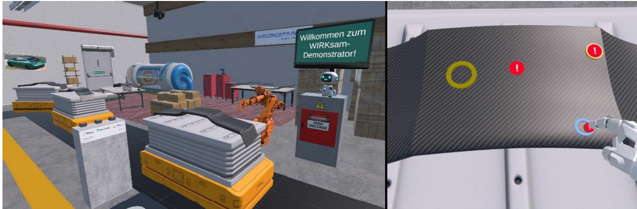
Figure 19: Left: Overview of the environment. Wings are transported by driverless systems, and a robotic arm is used to rotate the wings; the user controls these functions using buttons on the left. The robot and information display are visible on the right side of the image. Right: Illustration of how users mark defects. The yellow circles indicate defects detected by the AI system.
