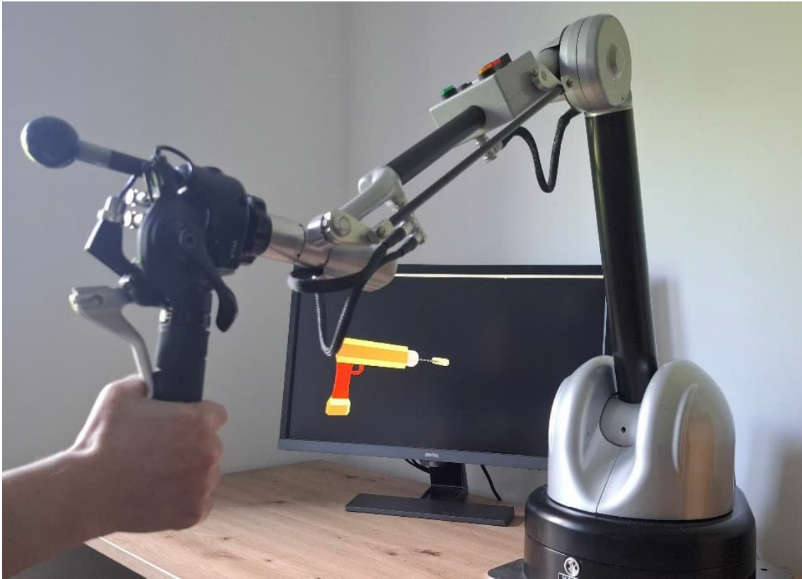
Figure 16. Second author testing the haptic rendering (without physical prop).
