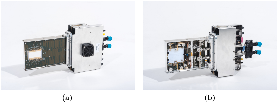
Fig. 1.14 Picture of an assembled station looking at the sensor side (a) and at the cooling side (b) [26].
