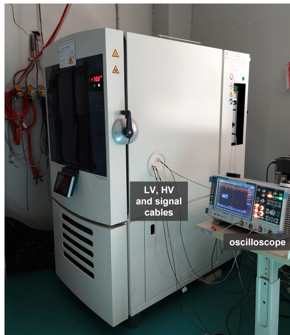
Fig. 8.1 Climatic chamber used for the characterization of the irradiated TimeSPOT sensors in laboratory. The Rohde & Schwarz RTO1044 oscilloscope used for the data acquisition is also visible.
