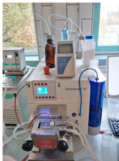
Fig. 1. Farinograph unit employed at the University of Hohenheim for the experimental part of this study.
