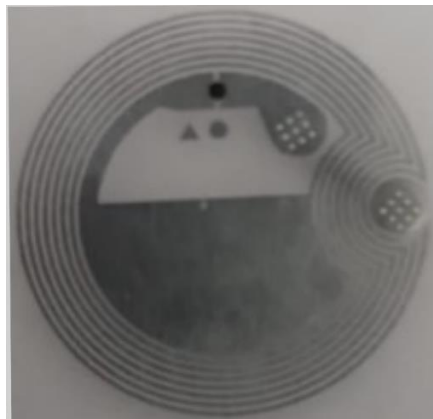
Fig. 1. HF RFID tag used for the characterization of the OS-based compound.
