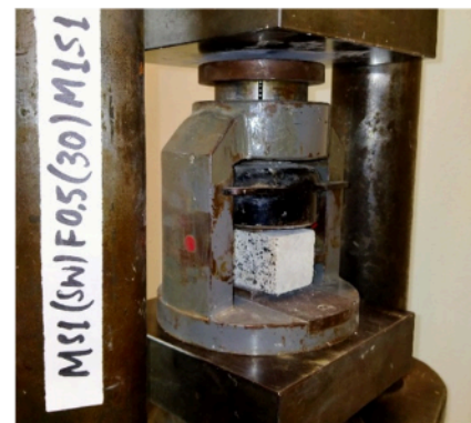
Fig. 4 Jute fiber composite mortar "MS1(SW)F0.5(30)M1S1" compressive strength test
