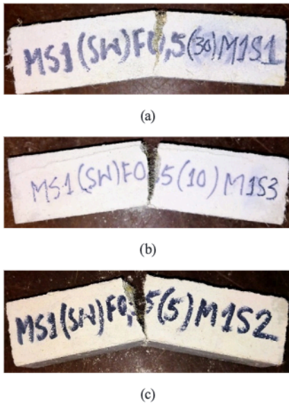
Fig. 5 Jute fiber composite mortar samples: (a) MS1(SW)F0.5(30)M1S1; (b) MS1(SW)F0.5(10)M1S3; and (c) MS1(SW)F0.5(5)M1S2 after the flexural strength test failures
