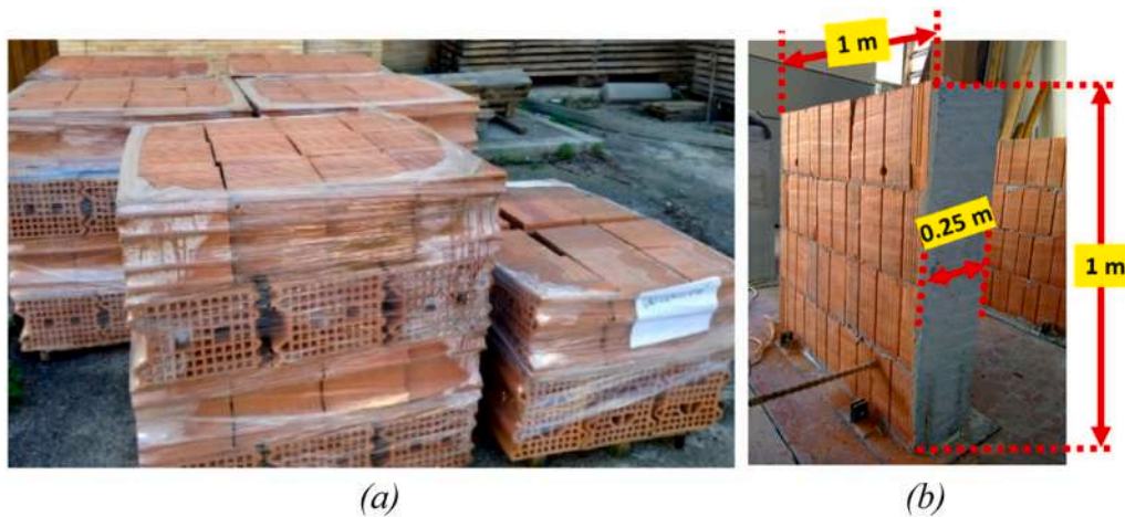
Fig. 9. (a) Hollow bricks, and (b) reference wall sample (1 m x 1 m x 0.25 m).
