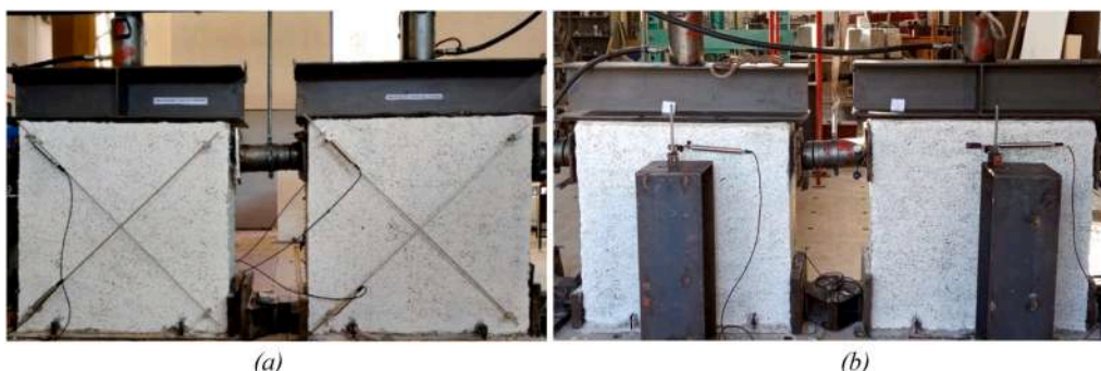
Fig. 15. Samples equipped at the (a) front with diagonal sensors and (b) back with horizontal sensors.
