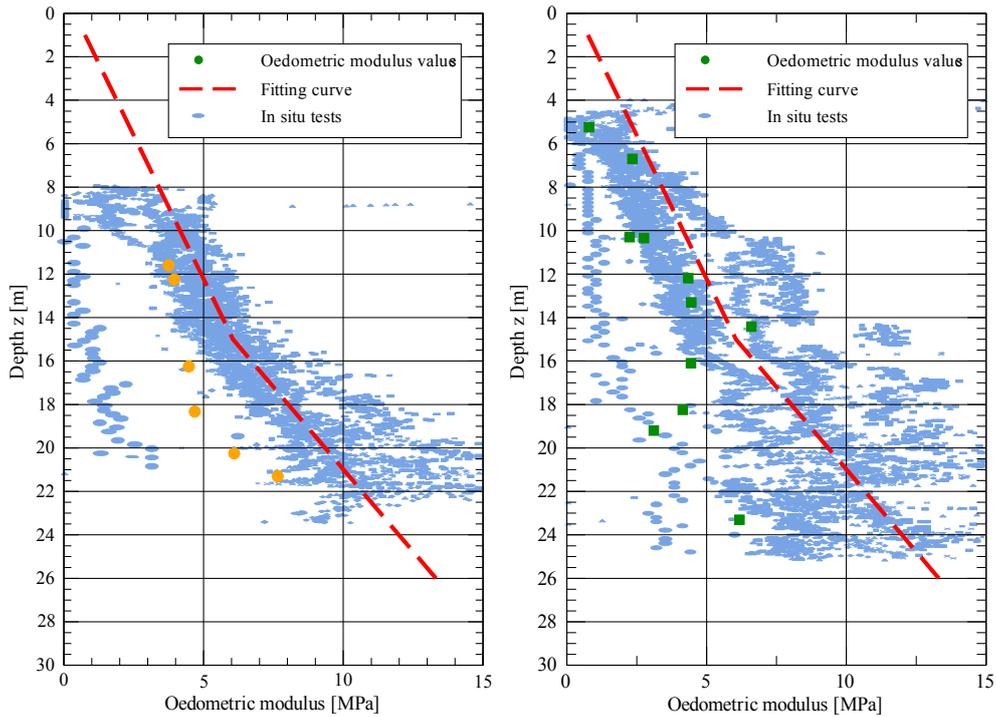
Figure 7. Trend of the oedometric modulus within the basin (CPTU test and oedometer test). Left: borehole A; Right: borehole B
