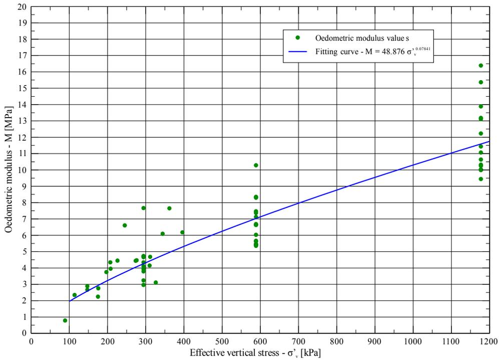
Figure 8. Evolution of the oedometric modulus as a function of the effective vertical stress ( $\sigma'_v$ )
