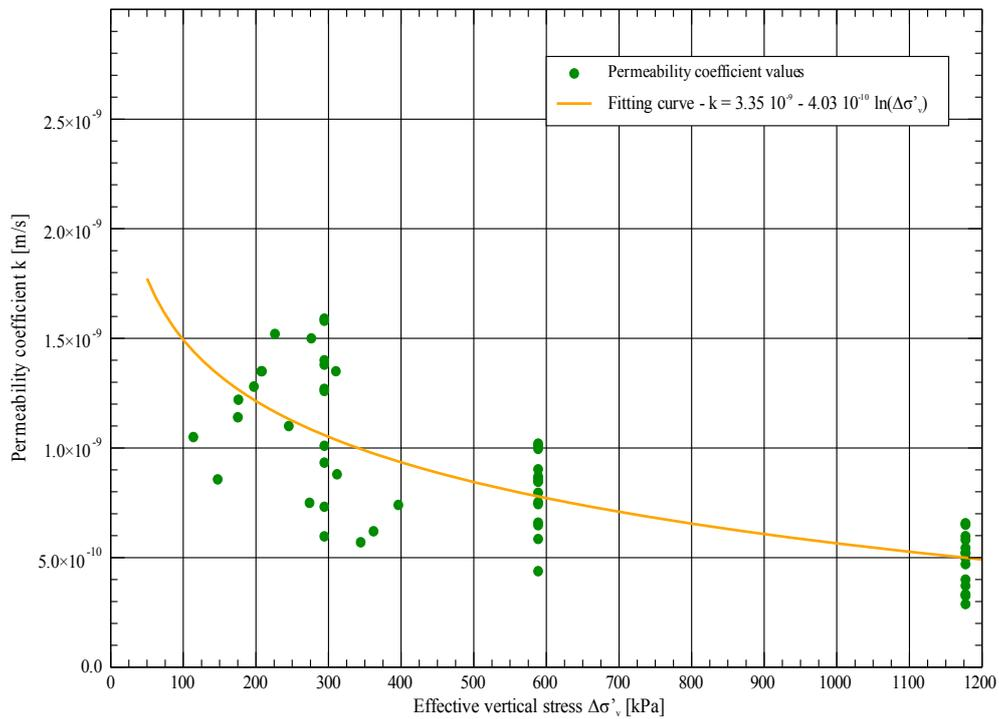
Figure 6. Trend of the permeability coefficient  $k$  as a function of the effective vertical stress  $\sigma'_v$
