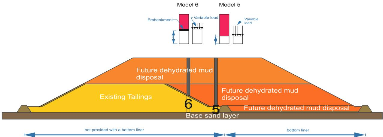
Figure 4. Section B of the basin with the indication of the calculus models
