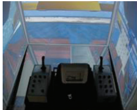
Fig. 1. Photo of (traditional) dynamic cockpit and graphic interface of the quay crane simulator.
